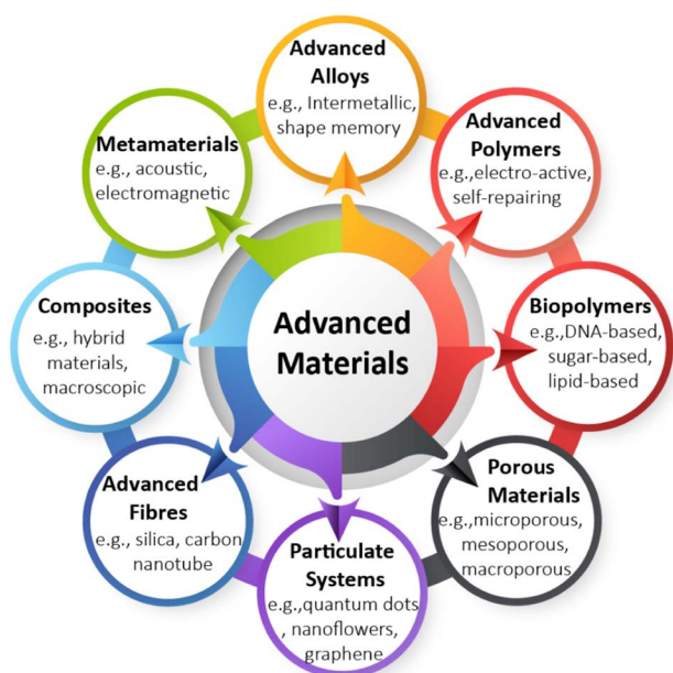
Fig. 1 Clusters of advanced materials proposed by the German Environment Agency (modified after Giese et al. 2020) based upon their physicochemical properties and structure. This classification does not distinguish the active and passive form of the AdMas, or how the physicochemical properties relate to the hazard.
