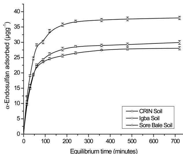
Fig. 5 Adsorption kinetics of  $\alpha$ -endosulfan on three different cocoa farm soils.
