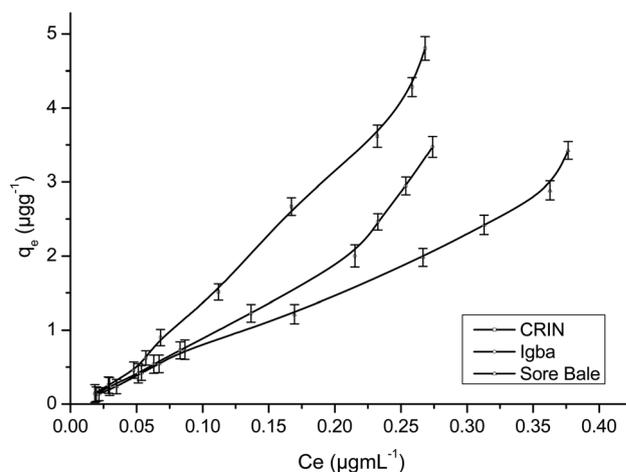
Fig. 11 Desorption isotherms of  $\alpha$ -endosulfan for CRIN, Igba and Sore Bale farm soils, where  $q_e$  = concentration of  $\alpha$ -endosulfan under-sorbed at equilibrium ( $\mu\text{g g}^{-1}$ ),  $C_e$  = concentration of  $\alpha$ -endosulfan desorbed into 0.01 M  $\text{CaCl}_2$  at equilibrium ( $\mu\text{g mL}^{-1}$ ).
