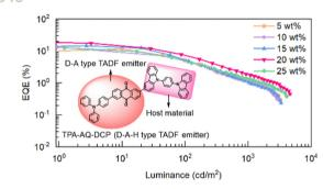
Asymmetric donor-acceptor-host red thermally activated delayed fluorescent emitter for high-efficiency organic light emitting diodes
