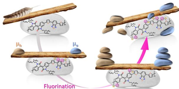
**The fluorination effect: the importance of backbone planarity in achieving high performance ambipolar field effect transistors**
