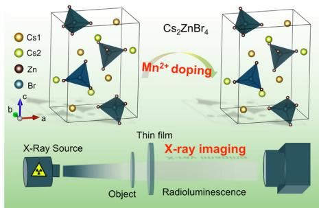
**Mn<sup>2+</sup>-doped Cs<sub>2</sub>ZnBr<sub>4</sub> scintillator for X-ray imaging**
