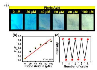
Fig. 5 (a) Digital images of TF-CD@PVDF films after adding different concentrations of PA (under UV illumination of 365 nm), (b) linearity plot of  $F_0/F$  vs. PA concentrations for TF-CD@PVDF composite films and (c) recyclability study of composite films for PA detection.
