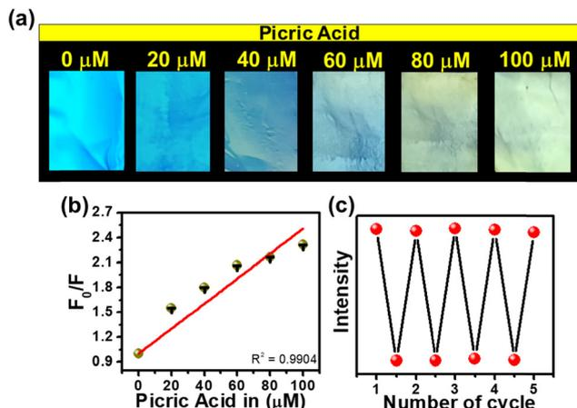
Fig. 5 (a) Digital images of TF-CD@PVDF films after adding different concentrations of PA (under UV illumination of 365 nm), (b) linearity plot of  $F_0/F$  vs. PA concentrations for TF-CD@PVDF composite films and (c) recyclability study of composite films for PA detection.
