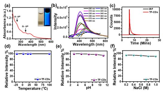
Fig. 2 (a) UV-vis spectra (inset: TF-CDs solution in both visible and UV light), (b) FL emission spectra and (c) TCSPC measurement recorded for TF-CDs. Stability plots of TF-CDs at different: (d) temperatures, (e) pH and (f) NaCl concentrations
