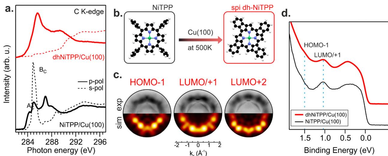
**Fig. 1** C K-edge NEXAFS spectra of the NiTPP monolayer deposited on the Cu(100) substrate kept at room temperature (black curves) and 500 K (red curves) during deposition (a); schematic representation of the reaction taking place on the copper surface held at 500 K (b); POT-based attribution of the frontier orbitals (c); valence band spectrum of NiTPP monolayer deposited on the Cu(100) substrate kept at room temperature (black curve) and 500 K (red curve) during deposition (d).
