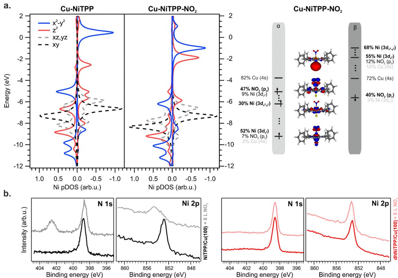
Fig. 5 DFT-calculated Ni pDOS for NiTPP-Cu and Cu-NiTPP- $\text{NO}_2$  (a). The different Ni 3d levels are colour coded as indicated by the legend (left); frontier energy levels of the optimized HS Cu-NiTPP- $\text{NO}_2$  cluster (right); experimental N 1s and Ni 2p core level spectra recorded on NiTPP/Cu(100) (black curve) and on dhNiTPP/Cu(100) (red curve) before and after exposure to  $\text{NO}_2$  (b).
