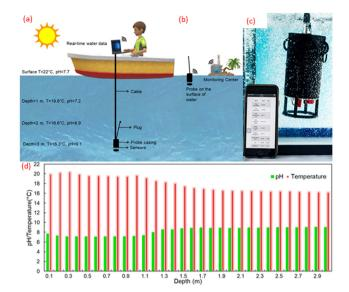
Fig. 8 (a) Features of the probe and changes in the temperature and pH of Großer Müggelsee lake with the depth (b) wireless communication of the quality of surface water to land (c) demonstration of the submergibility of the probe and the web server displaying water data on a phone (d) changes in temperature and pH every 0.1m from the surface.
