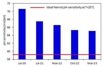
Fig. 9 pH sensitivity of fabricated electrodes over 32 months.
