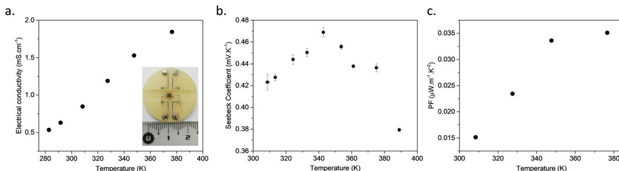
Fig. 2 (a) Temperature dependence of the electrical conductivity measured on a  $[\text{Cu}_2(1,3\text{-BDT})]_n$  pressed pellet by surface four-probe configuration and photo of the device to apply the bulk measurement of the electrical conductivity; (b) Seebeck coefficient with temperature (errors come from the linear fits of the raw data) and (c) the power factor with temperature.
