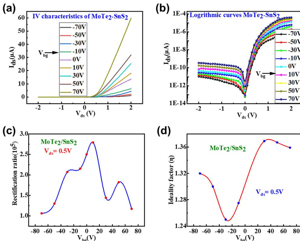
Fig. 4 (a)  $I_{ds}$ - $V_{ds}$  characteristic curves of the MoTe<sub>2</sub>-SnS<sub>2</sub> heterostructure at various back gate voltages ( $V_{bg}$ ); the linear scale. (b) Logarithmic scale. The maximum rectification ratio is  $2.79 \times 10^5$  mA W<sup>-1</sup>. (c) The change in the rectification ratio of the device at various back gate voltages. (d) The variation in the ideality factor at different gate voltages.
