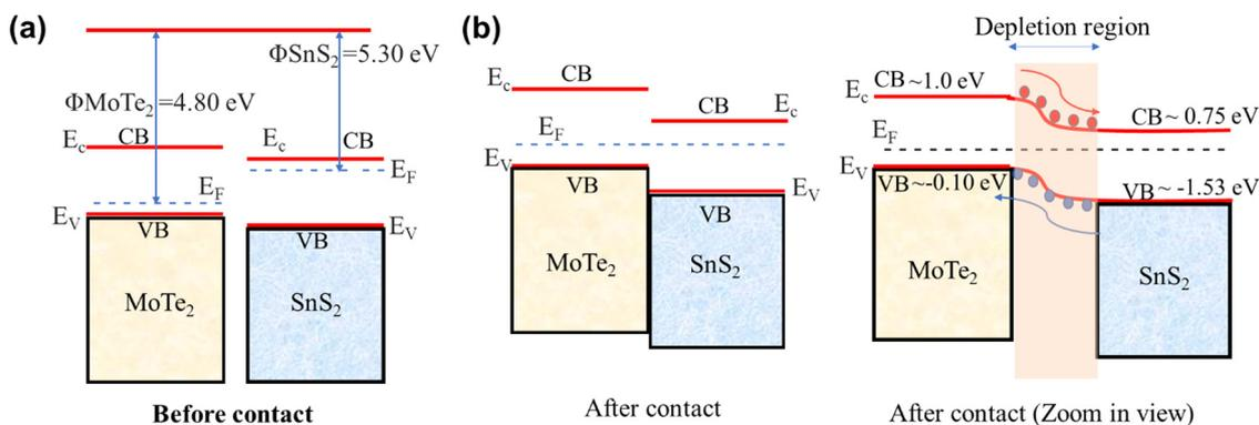
Fig. 5 Schematic illustration of the band diagram for the p-MoTe<sub>2</sub>/n-SnS<sub>2</sub> structure-based diode at  $V_{bg} = 0$  V. (a) Schematic signifies the band diagram of a p-MoTe<sub>2</sub>/n-SnS<sub>2</sub> diode before connection, and (b) symbolizes the diode after connection.
