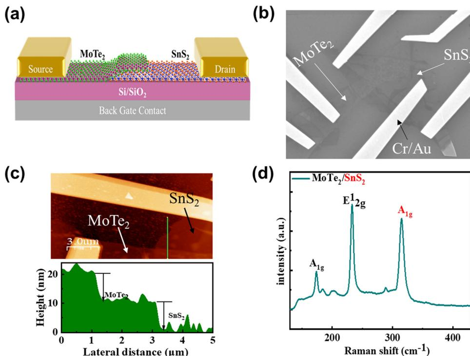
Fig. 1 (a) Schematic illustration of the p-n device. (b) SEM image of the p-n heterostructure MoTe<sub>2</sub>-SnS<sub>2</sub>-based device; the scale bar is 5 μm. (c) AFM profile of the heterostructure. (d) Raman spectra of the MoTe<sub>2</sub>-SnS<sub>2</sub> heterostructure.
