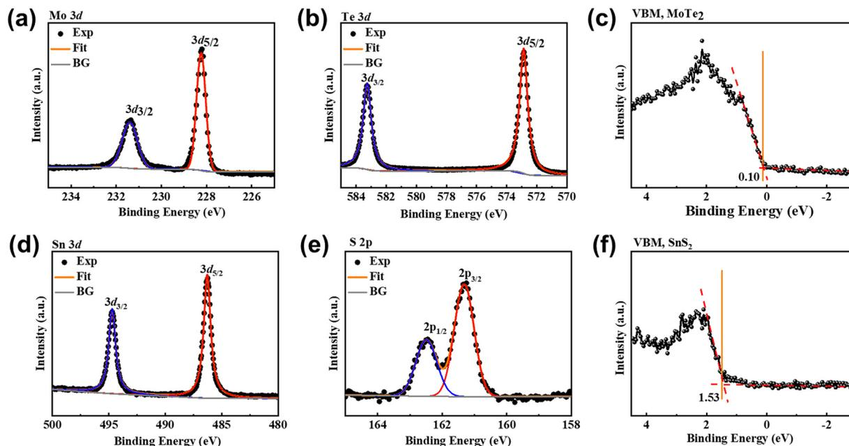
Fig. 3 XPS spectra: (a) Mo 3d peaks. (b) Te 3d peaks. (c) VBM of MoTe<sub>2</sub>. (d) Sn 3d peaks. (e) S 2p peaks. (f) VBM of SnS<sub>2</sub>.
