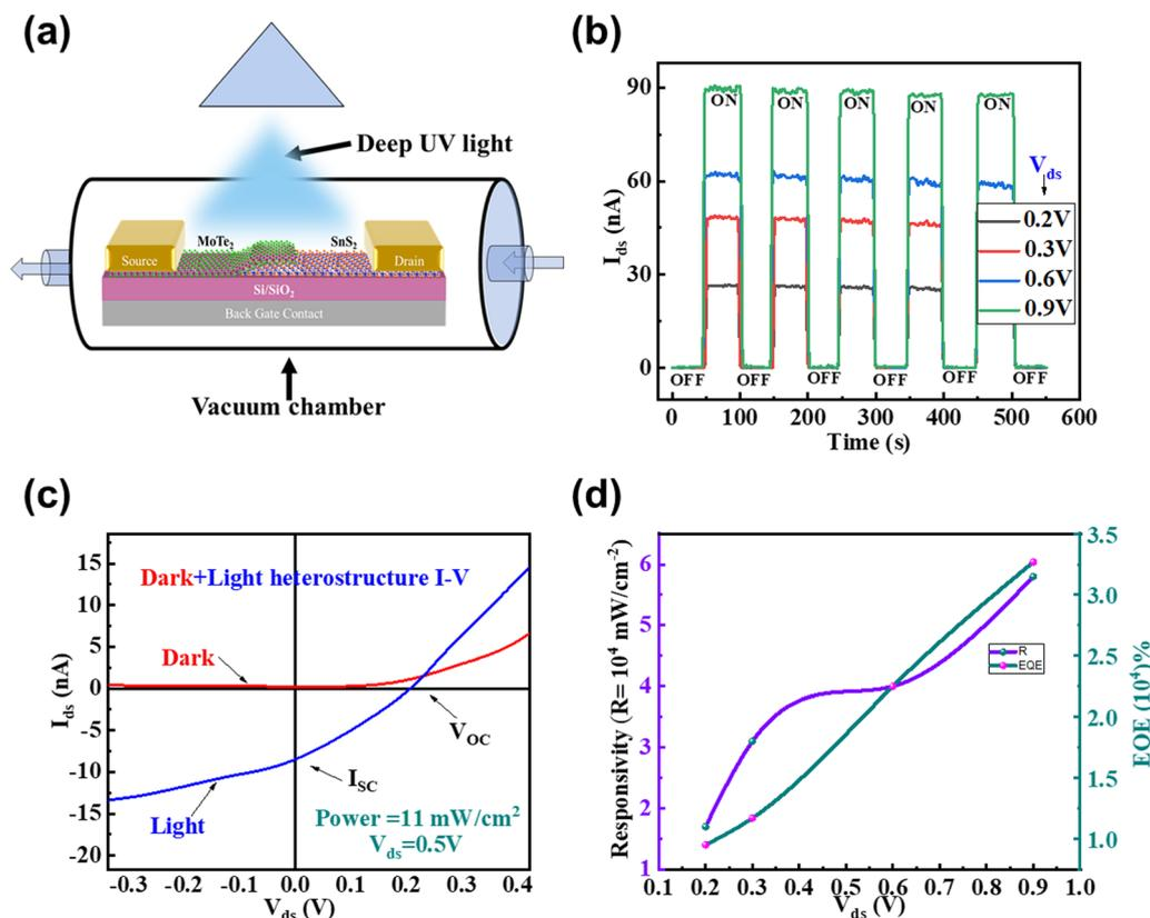
Fig. 6 (a) Schematic of the p–n device for photodetection. (b) Photocurrent at  $V_g = 0$ , for  $V_{ds} = 0.2$ – $0.9$  V with incident light ( $\lambda = 220$  nm) and power intensity 11 mA cm<sup>-2</sup>. (c)  $I$ – $V$  curves in the dark and under light, representing  $I_{sc} = -8.5$  nA and  $V_{oc} = 0.20$  V at  $V_g = 0$ . (d) The change in responsivity at different values of  $V_{ds}$ . (e) The enhancement in the EQE at different values of  $V_{ds}$ .
