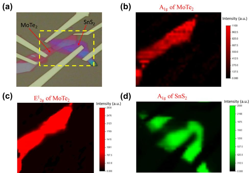
Fig. 2 (a) Optical image of the device that shows the area selected for Raman mapping. (b) Raman intensity maps of A<sub>1g</sub> of MoTe<sub>2</sub>. (c) Raman intensity maps of E<sub>1-2g</sub> of MoTe<sub>2</sub>. (d) Raman intensity maps of A<sub>1g</sub> of SnS<sub>2</sub>. Graphical representation of Raman intensity mapping at 172.43 and 232.93 cm<sup>-1</sup> for MoTe<sub>2</sub>, and 315.78 cm<sup>-1</sup> for SnS<sub>2</sub>.
