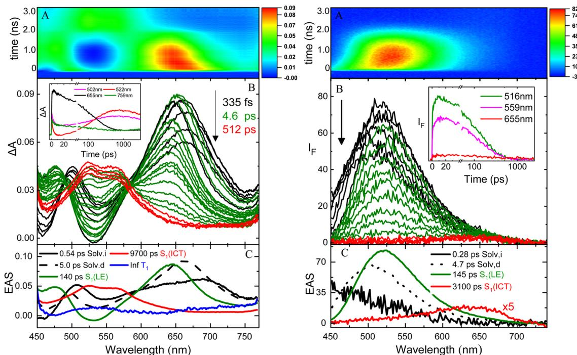
**Fig. 3** Femtosecond transient absorption (left) and broadband fluorescence up conversion spectroscopy (right) of **NPI-Ph-PTZ** in toluene with a 400 nm laser excitation (panel A:  $\Delta A/I_F$  vs. wavelength and time colored map; panel B: time resolved absorption/emission spectra and kinetics at selected wavelengths (inset); panel C: Evolution Associated Spectra (EAS) and lifetimes of the components obtained through global analysis).
