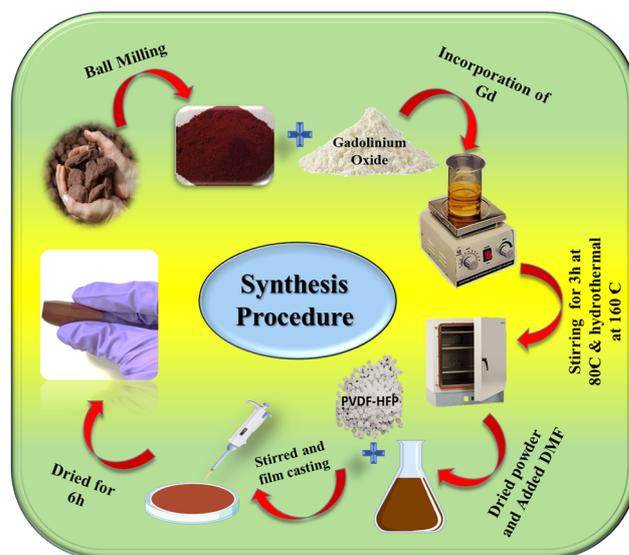
Scheme 1 Schematic representation of the synthesis procedure.
