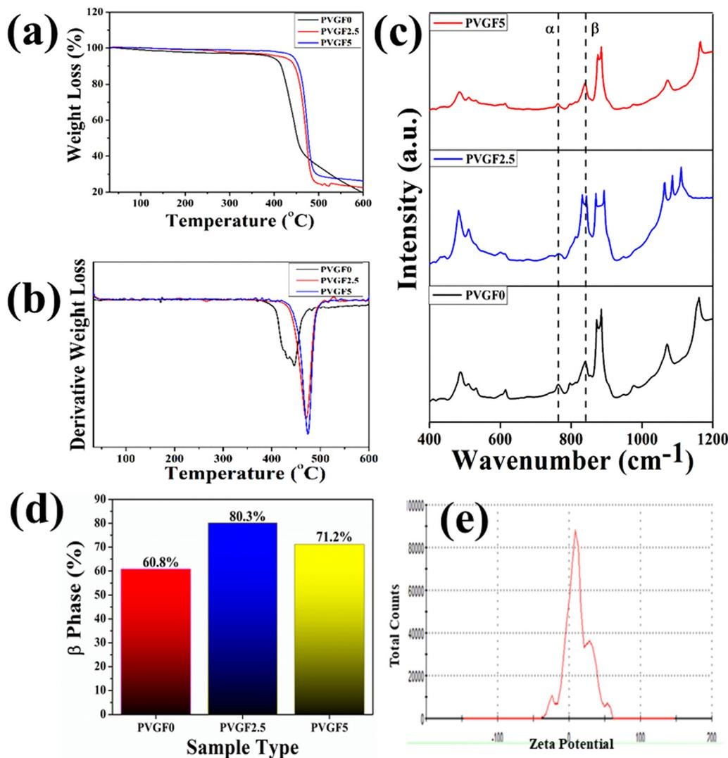
**Fig. 3** (a) Percentage weight losses of nanocomposite membranes. (b) Derivative weight loss of the nanocomposite membranes, suggesting better stability in doped membranes. (c) FTIR spectroscopy of PVGF0, PVGF2.5, and PVGF5, showing polar phase enhancement after nanocomposite inclusion into the polymer matrix. (d) Percentage  $\beta$ -phase of samples PVGF0, PVGF2.5, and PVGF5. (e) The zeta potential of Gd-incorporated hematite shows a high positive surface charge.
