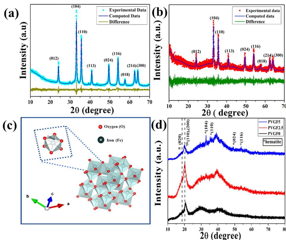
Fig. 1 (a) and (b) Experimental and computed XRD patterns of natural  $\alpha$ -hematite and Gd-incorporated  $\alpha$ -hematite, respectively. (c) Unit cells of Gd-incorporated  $\alpha$ -hematite. (d) XRD patterns of natural Gd-incorporated  $\alpha$ -hematite nanocomposite membranes suggesting that incorporation of nanocomposite into the polymer matrix enhances the polar phase, finding a maximum in PVGF2.5.
