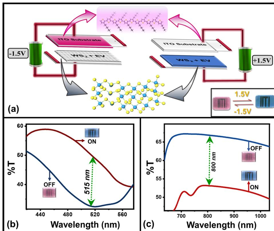
Fig. 2 (a) Schematic representation of the layered device along with its actual photographs (inset) under different bias conditions, (b) *in situ* bias dependent transmission spectra of the device in the visible ( $\sim 515$  nm) as well as NIR ( $\sim 800$  nm) wavelength region in (c). Graphics Partly adopted with permission from ref. 26 Copyright American Chemical Society (2023).
