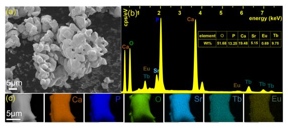
Fig. 2 SEM image of  $Ca_8SrTb(PO_4)_7:0.1Eu^{2+}$  (a), EDS spectra and mass ratio of elements of  $Ca_8SrTb(PO_4)_7:0.1Eu^{2+}$  (b), and elemental mappings of  $Ca_8SrTb(PO_4)_7:0.1Eu^{2+}$  phosphors (c).
