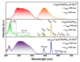
Fig. 4 PL and PLE spectra of Ca<sub>8</sub>SrGd(PO<sub>4</sub>)<sub>7</sub>:0.1Eu<sup>2+</sup>, Ca<sub>8</sub>SrTb(PO<sub>4</sub>)<sub>7</sub>: 0.1Eu<sup>2+</sup> and Ca<sub>8</sub>SrTb(PO<sub>4</sub>)<sub>7</sub> phosphors.
