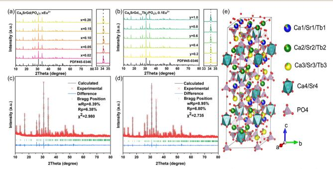
Fig. 1 XRD patterns ( $2\theta = 10 - 80^{\circ}$ ) and enlarged XRD patterns at  $2\theta = 33 - 35.3^{\circ}$  of the Ca<sub>8</sub>SrGd(PO<sub>4</sub>)<sub>7</sub>:XEu<sup>2+</sup> (a) and Ca<sub>8</sub>SrGd(PO<sub>4</sub>)<sub>7</sub>:0.1Eu<sup>2+</sup>, yTb<sup>3+</sup> (b), the Rietveld refinement results of  $Ca_8SrGd(PO_4)_7$  (c) and  $Ca_8SrTb(PO_4)_7$ :0.1Eu<sup>2+</sup> (d), and the crystal structure of  $Ca_8SrTb(PO_4)_7$ :0.1Eu<sup>2+</sup> (e).
