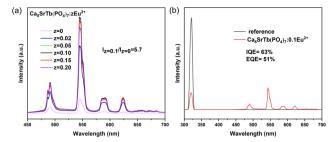
Fig. 6 (a) PL spectra of phosphor  $Ca_8SrTb(PO_4)_7$ : $zEu^{2+}$  (z=0, 0.02, 0.05, 0.10, 0.15, and 0.20) at 365 nm excitation. (b) IQE and EQE of phosphor  $Ca_8SrTb(PO_4)_7$ :0.1Eu<sup>2+</sup> at 320 nm excitation.
