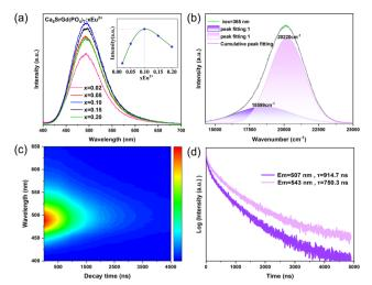
Fig. 3 (a) PL spectra of  $Ca_8SrGd(PO_4)_7$ :  $xEu^{2+}(x = 0.02, 0.05, 0.10, 0.15, 0.10, 0.15)$ and 0.20) phosphors excited at 365 nm and the inset shows the change of intensity with Eu<sup>2+</sup> concentration. (b) Gaussian fitting results of the PL spectrum of  $Ca_8SrGd(PO_4)_7:0.1Eu^{2+}$  phosphors. (c) TRPL of  $Ca_8SrGd$ (PO<sub>4</sub>)<sub>7</sub>:0.1Eu<sup>2+</sup>. (d) Decay curves of the emissions of Ca<sub>8</sub>SrGd  $(PO_4)_7:0.1Eu^{2+}$  at 507 and 543 nm.
