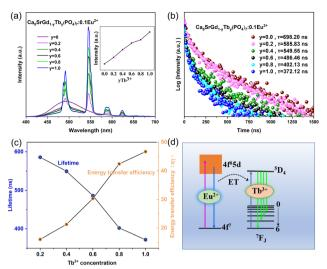
Fig. 5 (a) PL spectra of phosphor  $Ca_8SrGd(PO_4)_7:0.10Eu^{2+}$ ,  $yTb^{3+}$  at 365 nm excitation and the inset shows the change of intensity with the  $Tb^{3+}$  concentration. (b) Decay curves of the emission from  $Ca_8SrGd(PO_4)_7:0.1Eu^{2+}$ ,  $yTb^{3+}$  at 450 nm. (c) Changes of energy transfer efficiency and lifetime with increasing concentration of Tb ions in  $Ca_8SrGd(PO_4)_7:0.10Eu^{2+}$ ,  $yTb^{3+}$ . (d) Energy transfer diagram.
