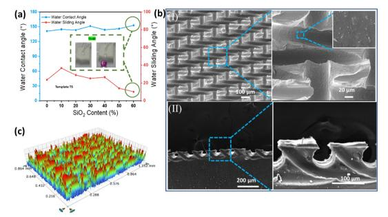
Fig. 2 (a) Dependence of the water contact and sliding angles of the stretchable PDMS elastomer formed by template TS on the SiO<sub>2</sub> content, with images of the self-cleaning test for the TS-60 sample (SiO<sub>2</sub> content: 60%) shown in the inset. (b) Top (top) and cross-sectional (bottom) views of the SEM images of TS-60. (c) Three-dimensional (3D) profile image of TS-60 for an area of 1 mm  $\times$  1 mm.
