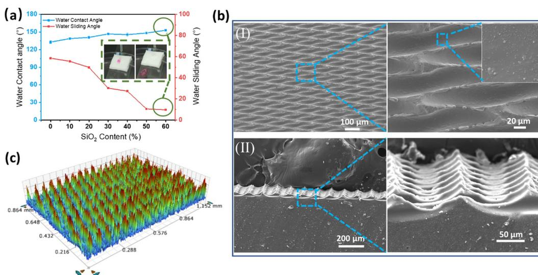
Fig. 3 (a) Dependence of the water contact and sliding angles of the stretchable PDMS elastomer formed by the template TW on the SiO<sub>2</sub> content, with images of the self-cleaning test for the TW-60 sample shown in the inset. (b) Top (top) and cross-sectional (bottom) views of the SEM images of TW-60. (c) 3D profile image of TW-60.
