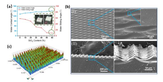
Fig. 3 (a) Dependence of the water contact and sliding angles of the stretchable PDMS elastomer formed by the template TW on the SiO<sub>2</sub> content, with images of the self-cleaning test for the TW-60 sample shown in the inset. (b) Top (top) and cross-sectional (bottom) views of the SEM images of TW-60. (c) 3D profile image of TW-60
