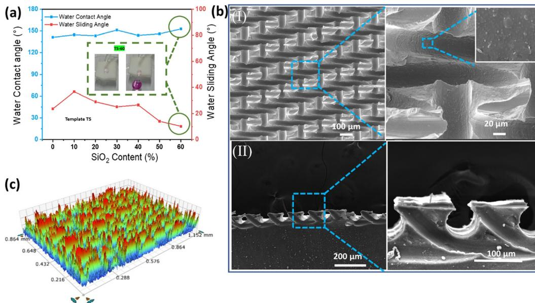
Fig. 2 (a) Dependence of the water contact and sliding angles of the stretchable PDMS elastomer formed by template TS on the SiO<sub>2</sub> content, with images of the self-cleaning test for the TS-60 sample (SiO<sub>2</sub> content: 60%) shown in the inset. (b) Top (top) and cross-sectional (bottom) views of the SEM images of TS-60. (c) Three-dimensional (3D) profile image of TS-60 for an area of 1 mm × 1 mm.
