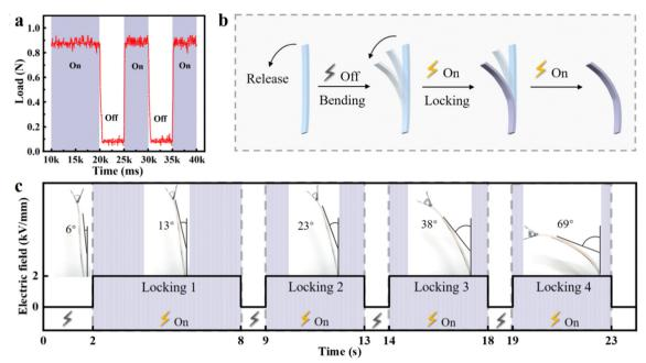
Fig. 6 Response time and motion locking of the ER structure. (a) Response time and repeatability of the structure. (b) Schematic of the principle of motion locking. (c) Demonstration of the locking behavior of the soft structure
