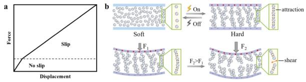
Fig. 4 Principle of the forces affecting the ER particle chains during the deformation. (a) Process division during deformation. (b) Microstructure schematic of the variation in stiffness, and the way applied force destroys the particle chains during deformation.
