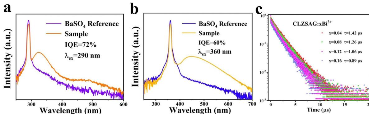
Fig. 5 (a) IQE of the CLZSAG:0.06Bi<sup>3+</sup> phosphor under 290 nm excitation. (b) IQE of the CLZSAG:0.14Bi<sup>3+</sup> phosphor under 360 nm excitation. (c) PL decay curves of CLZSAG:xBi<sup>3+</sup> at room temperature ( $\lambda_{\text{ex}} = 375$  nm,  $\lambda_{\text{em}} = 467$  nm).
