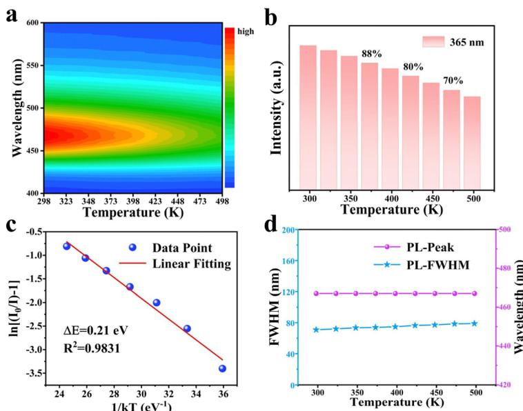
Fig. 6 (a) Contour maps of the emission spectra of the temperature variation of CLZSAG:0.14Bi<sup>3+</sup> ( $\lambda_{\text{ex}} = 365$  nm). (b) Normalized integrated intensity with temperature for CLZSAG:0.14Bi<sup>3+</sup>. (c) Linear fittings of the relationship between  $\ln(I_0/I) - 1$  with a  $1/kT$  of CLZSAG:0.14Bi<sup>3+</sup>. (d) The temperature-dependent of the PL peak position and FWHM.
