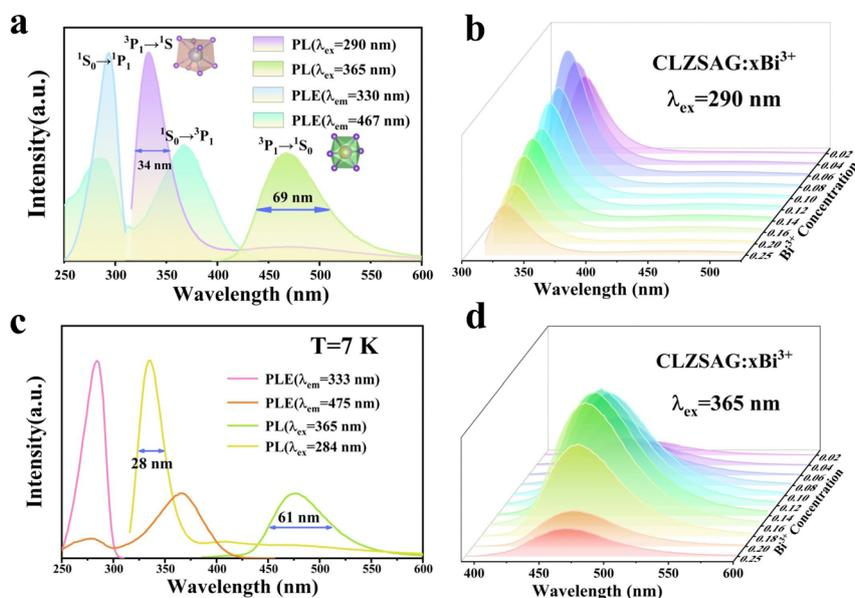
Fig. 4 (a) PLE and PL spectra of CLZSAG:0.14Bi<sup>3+</sup>. (b) The PL spectra of CLZSAG:xBi<sup>3+</sup> (0.02 ≤ x ≤ 0.25) under the excitation of 365 nm. (c) The emission spectrum of the CLZSAG:Bi<sup>3+</sup> phosphor measured at 10 K. (d) The PL spectra of CLZSAG:xBi<sup>3+</sup> (0.02 ≤ x ≤ 0.25) under the excitation of 290 nm.
