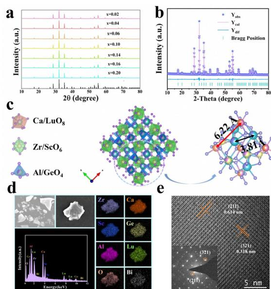
Fig. 1 (a) XRD patterns of the CLZSAG:*x*Bi<sup>3+</sup> samples ( $2\theta = 10\text{--}80^\circ$ ). (b) Rietveld refinement of CLZSAG:0.04Bi<sup>3+</sup>. (c) Crystal structure of CLZSAG. (d) SEM images, EDS spectrum and elemental maps of the CLZSAG:0.14Bi<sup>3+</sup> sample. (e) High-resolution TEM (HRTEM) images of the CLZSAG:0.14Bi<sup>3+</sup> sample; the inset shows the selected area electron diffraction patterns.
