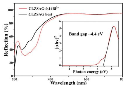
**Fig. 2** DR spectra of the CLZSAG host and CLZSAG:0.14Bi<sup>3+</sup> phosphors (the inset shows the calculated optical band gap values of the CLZSAG host based on the DR spectra).
