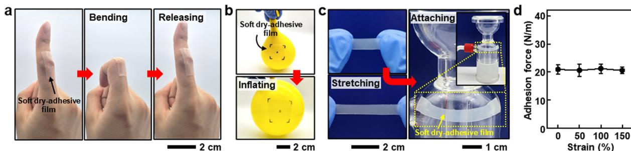
Fig. 5 Various adhesive properties of the soft dry-adhesive film. (a–c) Optical images of the 2.5 wt% Tween 80-added soft dry-adhesive film (a) stretched on a human finger, (b) inflated on a rubber balloon, and (c) stretched and then attached to a glass object. (d) Adhesion forces of the 2.5 wt% Tween 80-added soft dry-adhesive film when stretched by specific mechanical strains and attached to dry human skin ( $n = 5$ ).
