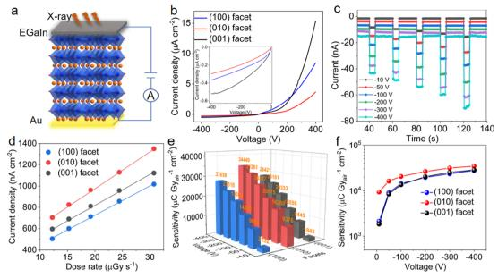
Fig. 4 (a) Schematic diagram of the CsPbBr<sub>3</sub> detector structure. (b) J-V curves in dark from -400 V to 400 V. The inset shows the enlarged details from -400 V to 0 V. (c) Temporal X-ray responses of the device based on the (010) wafer under voltages from -10 V to -400 V. (d) Photocurrent response via dose rates at -400 V and (e and f) X-ray sensitivities of the (100), (010), and (001) wafers under different voltages.
