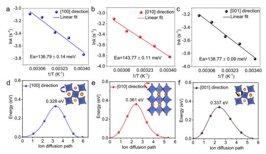
Fig. 3 (a-c) Ion migration activation energies of CsPbBr<sub>3</sub> crystal wafers along the [100], [010], and [001] directions, respectively. (d-f) Calculated energy profiles of different ionic migration paths for Br ion vacancy along the [100], [010], and [001] orientations.
