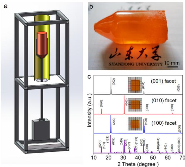
Fig. 1 (a) Schematic diagram of the vertical Bridgman furnace. (b) Photograph of an as-grown  $\text{CsPbBr}_3$  single crystal. (c) XRD patterns of the (100), (010), and (001) wafers. The insets are photographs of the processed and polished wafers.
