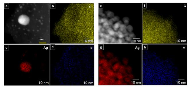
Fig. 2 (a-h) STEM elemental mapping of ATP: C, Ag, and O atoms indicating presence of infused silver nanoclusters in ATP.
