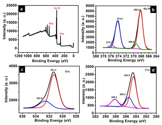
(a) XPS survey spectrum, (b) high-resolution XPS spectra of Ag 3d, (c) O1s, (d) C1s.
