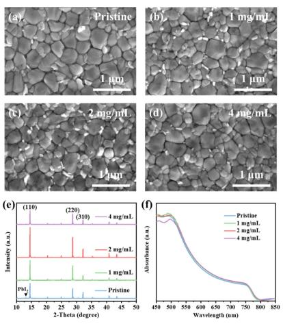
Fig. 1 (a)–(d) SEM images of perovskite films with different concentrations of TEAPF<sub>6</sub>. (e) XRD pattern and (f) UV-vis spectra of perovskite films with different concentrations of TEAPF<sub>6</sub>.
