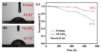
Fig. 5 (a) and (b) The water contact angle of perovskite films without and with TEAPF<sub>6</sub>. (c) The long-term stability of PSCs.
