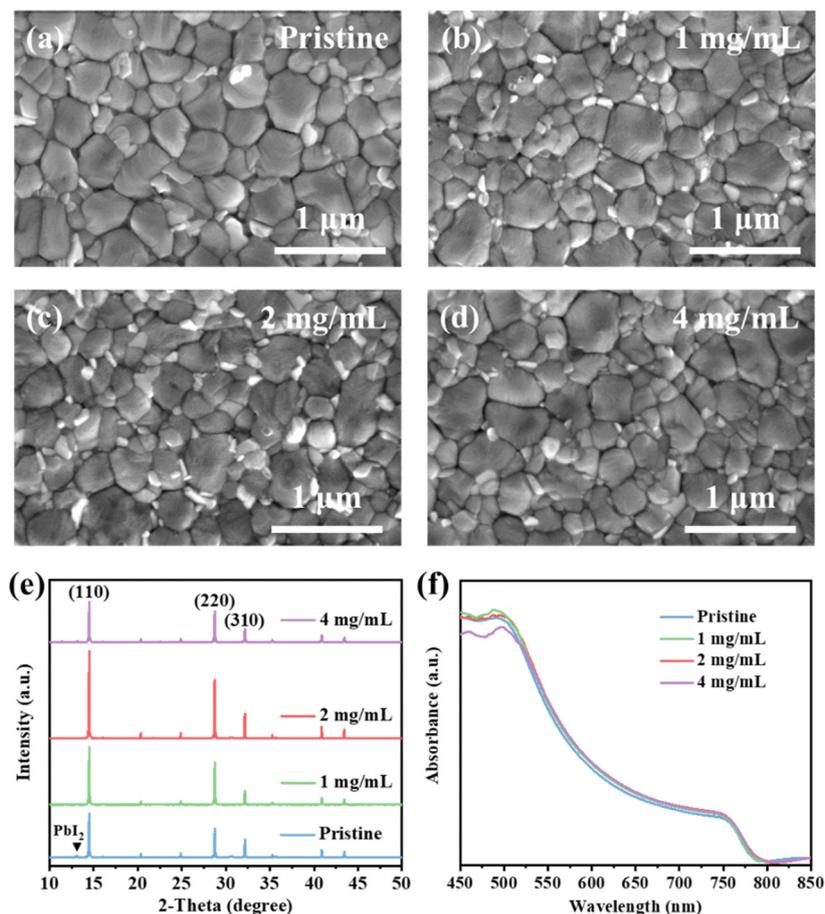
Fig. 1 (a)–(d) SEM images of perovskite films with different concentrations of TEAPF<sub>6</sub>. (e) XRD pattern and (f) UV-vis spectra of perovskite films with different concentrations of TEAPF<sub>6</sub>.
