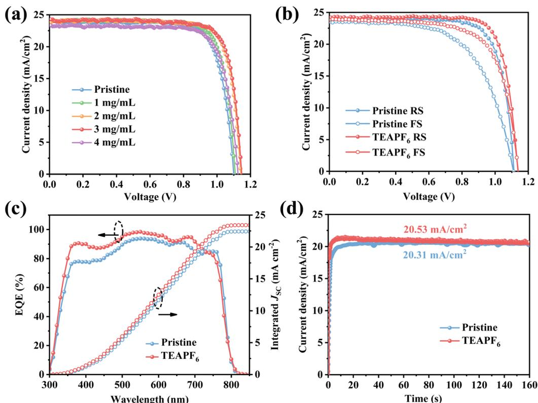
Fig. 3 (a)  $J$ - $V$  curves of PSCs with different concentrations of  $\text{TEAPF}_6$ . (b)  $J$ - $V$  curves in different scan directions. (c) EQE spectra and (d) steady-state output  $J_{\text{SC}}$  of PSCs.
