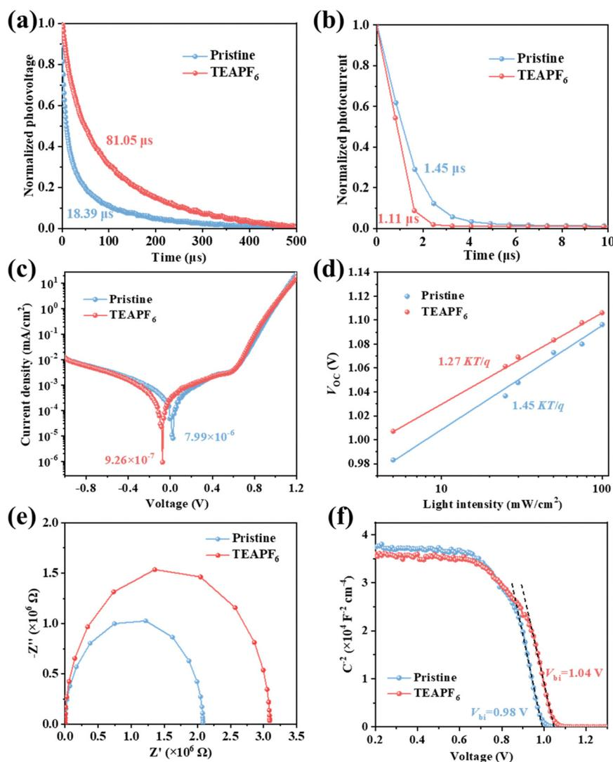
Fig. 4 (a) TPV and (b) TPC measurements, (c) dark  $J$ - $V$  measurements, (d)  $V_{OC}$  as a function of light intensity, (e) EIS measurements, and (f)  $C$ - $V$  measurements of the PSCs without and with TEAPF<sub>6</sub>.
