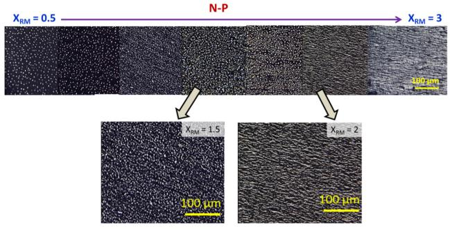
Fig. 2 POM images taken in the isotropic for samples polymerised in the nematic phase (N-P) for varied X<sub>RM</sub>. While droplet morphology is seen for lower  $X_{\rm RM}$ , as the monomer concentration increases, improved connectivity of the polymer fibres was observed. Enlarged images (below) display oriented polymer strands that are the resultant of the surrounding aligned nematic environment.
