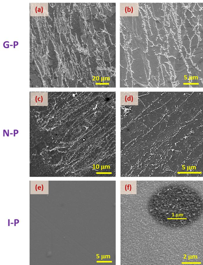
Fig. 5 SEM images depicting the polymer networks for  $X_{\text{RM}} = 1.75$  with magnifications, (a)  $1 \times 10^3$ , (b)  $5 \times 10^3$ , (c)  $2.5 \times 10^3$ , (d)  $7.5 \times 10^3$ , (e)  $5 \times 10^3$ , (f)  $15 \times 10^3$  for G-P, N-P and I-P samples shown from top to bottom, respectively. Inset in (f) showcases the short polymer strands at a higher magnification of  $30 \times 10^3$ .
