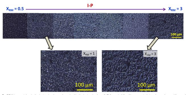
Fig. 3 POM images taken in the isotropic when polymerised in the isotropic phase (I-P) for varied  $X_{RM}$ . No connected strands are observed for any  $X_{RM}$ . even in enlarged images (shown below).
