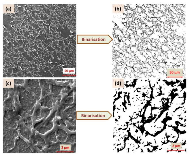
Fig. 8 Binarisation of the SEM images for  $X_{\text{RM}}=3$  in two different magnifications (500 and  $20\times10^3$ ) for the G-P case
