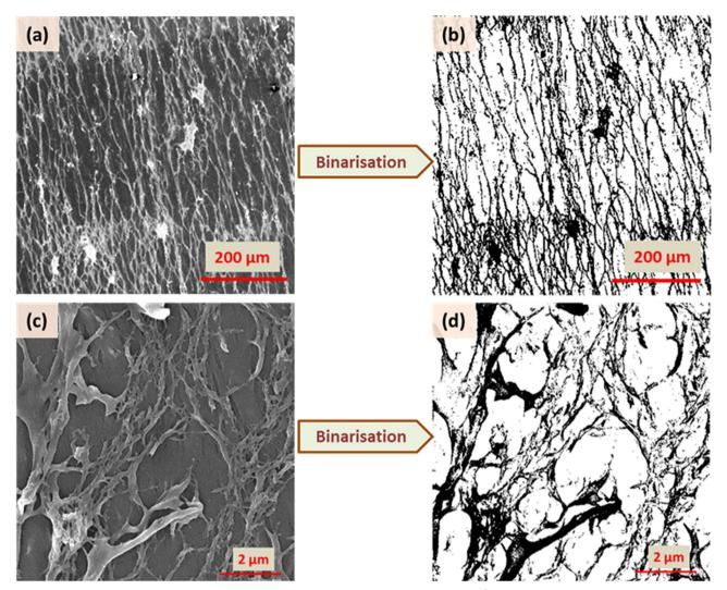
Fig. 7 Binarisation of the SEM images for  $X_{RM} = 3$  in two different magnifications (125 and 15  $\times$  10<sup>3</sup>) for the N-P case
