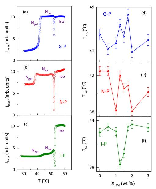
Fig. 10 Thermal variation of transmitted laser intensity ( $I_{laser}$ ) for the G-P, N-P, and I-P cases, for  $X_{RM} = 1$  in (a), (b), (c) respectively. The variation of  $T_{sg}$  with different  $X_{RM}$  is shown for the G-P, N-P, and I-P cases in (d), (e), (f), respectively.
