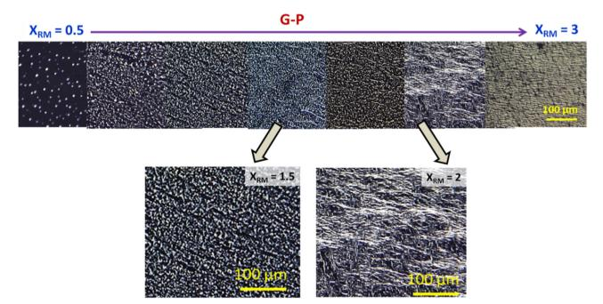
Fig. 1 POM images taken in the isotropic for samples polymerised in gel phase (G-P) with varied concentrations of photopolymer ( $X_{RM}$ ). Droplet morphology was seen for lower  $X_{RM}$ , and improved the connectivity of the polymer strands was observed with the increase in the monomer concentration. Although enlarged images (below) display well-connected polymer networks at higher  $X_{RM}$ , the networks are more distorted; a consequence of the surrounding nematic-gel environment.
