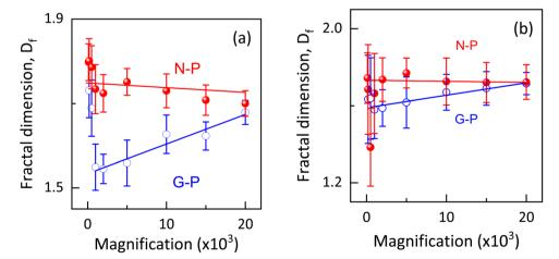
Fig. 9 Variation of fractal dimension  $D_f$  at different magnifications for N-P and G-P samples by open source software (a) ImageJ and (b) Fractalyse. In both tools, higher  $D_f$  is exhibited by the N-P compared to the G-P samples for all magnifications.
