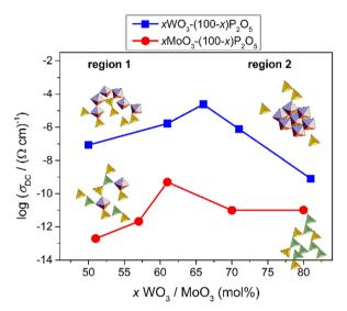
Fig. 4 Compositional dependence of DC conductivity at 303 K for  $xWO_3$ -(100–x)P $_2O_5$  and  $xMoO_3$ -(100–x)P $_2O_5$ , x=49-81 mol% glass series. Region 1 includes glass compositions up to the conductivity maximum with the 2D interconnection of TM units, whereas region 2 corresponds to the glass compositions above the conductivity maximum where the 3D interconnection of TM units occurs. The lines are drawn as a guide to the eye.
