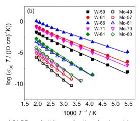
Fig. 3 (a) Conductivity spectra at different temperatures of the Mo-61 glass and (b) DC conductivity as a function of reciprocal temperature of phosphate glasses containing  $WO_3$  (solid symbols) and  $MoO_3$  (open symbols). The straight lines were obtained by linear regression. The error bars are at most of the order of the symbol size.
