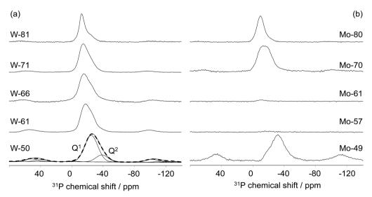
Fig. 2  $^{31}$ P MAS-NMR spectra of glasses from (a)  $xWO_3$ -(100-x)P<sub>2</sub>O<sub>5</sub> and (b)  $xMoO_3$ -(100-x)P<sub>2</sub>O<sub>5</sub>, x = 49-81 mol%, series.
