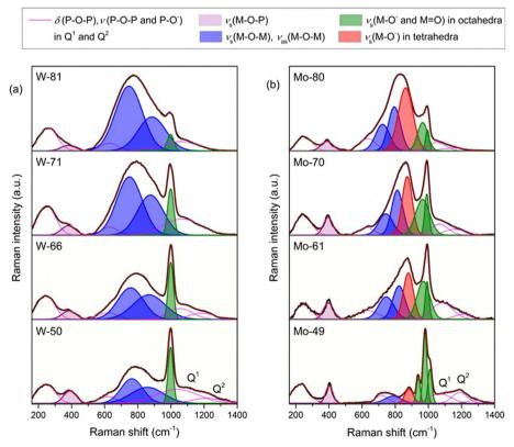
Fig. 1 Raman spectra of glasses from (a)  $xWO_3$ -(100-x) $P_2O_5$  and (b)  $xMoO_3$ -(100-x) $P_2O_5$ , x = 49-81 mol%, series. The Raman spectra of W-61 and Mo-57 are similar to those of W-66 and Mo-61, respectively; hence, they are not shown.
