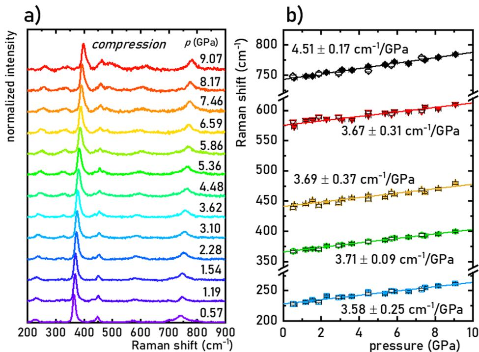
Fig. 2 Normalized Raman spectra for the SrGdAlO<sub>4</sub> material measured for different pressure values, during the compression cycle (a); determined energies (peak centroids) of the most intense phonon modes as a function of pressure (b); filled symbols represent compression data and empty ones represent decompression data; the continuous lines are the linear fits applied for determination of the pressure shift rates of the corresponding Raman modes.
