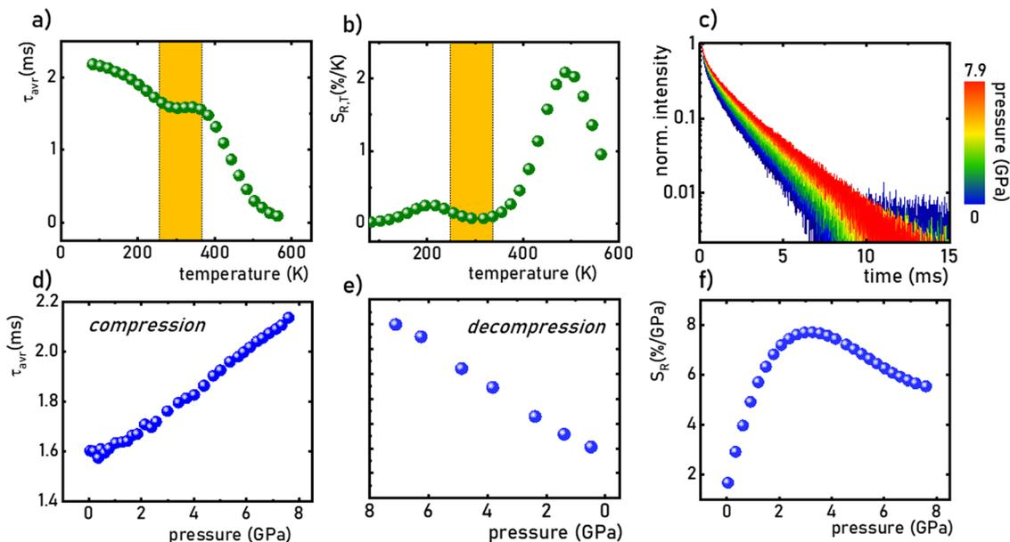
Fig. 5 The  $\tau_{avr}$  of the SrGdAlO<sub>4</sub>:0.2%Mn<sup>4+</sup> measured as a function of temperature (a) the corresponding  $S_{R,T}$  (b); luminescence decay profile of SrGdAlO<sub>4</sub>:0.2%Mn<sup>4+</sup> measured as a function of pressure (c); the  $\tau_{avr}$  measured at room temperature as a function of pressure during compression (d) and decompression (e) and corresponding  $S_{R,p}$  (f).
