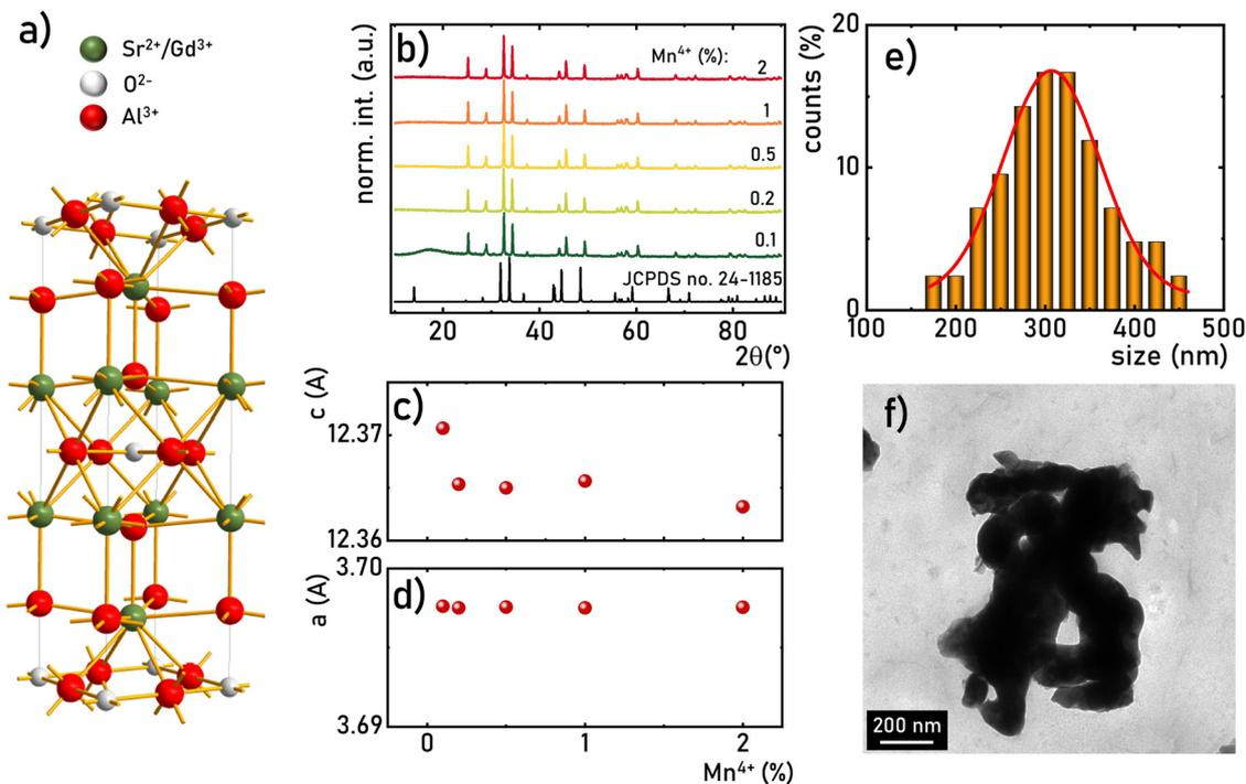
Fig. 1 Visualization of the crystal structure of the SrGdAlO<sub>4</sub> material (a); XRD patterns of the SrGdAlO<sub>4</sub>: Mn<sup>4+</sup> for different concentrations of dopant ions (b); calculated c (c) and a (d) parameters for the SrGdAlO<sub>4</sub>: Mn<sup>4+</sup> material as a function of Mn<sup>4+</sup> concentration; particle size distribution ( $d_{avr} = 306$  nm, FWHM = 98 nm) (e) and representative TEM image (f) of the SrGdAlO<sub>4</sub>:0.2%Mn<sup>4+</sup>.
