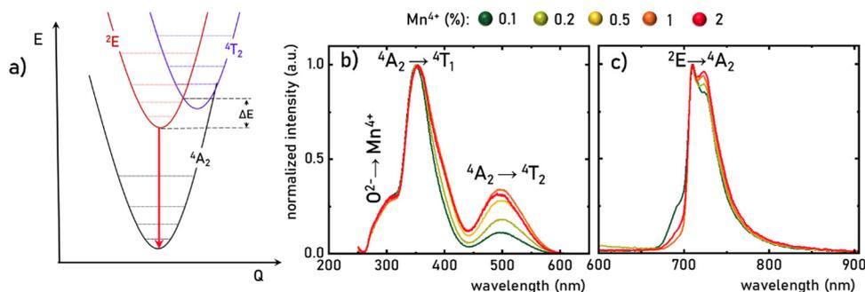
Fig. 3 Simplified configurational coordination diagram of Mn<sup>4+</sup> ions (a), the comparison of the normalized room temperature excitation spectra ( $\lambda_{\text{em}} = 710$  nm) (b), and emission spectra ( $\lambda_{\text{exc}} = 400$  nm) (c) of SrGdAlO<sub>4</sub>:Mn<sup>4+</sup> with different concentration of Mn<sup>4+</sup> ions.
