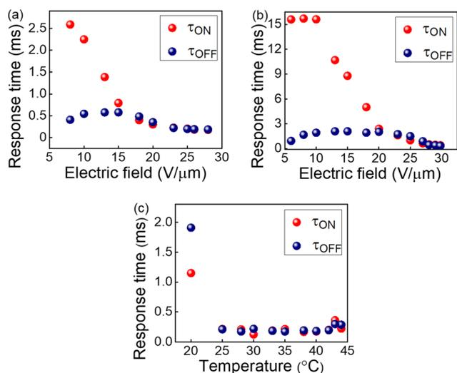
Fig. 5 Electric field dependence of response times in BPIII of the QD-BPLC at (a)  $35^\circ\text{C}$  and (b)  $25^\circ\text{C}$ . (c) Thermal dependence of response times at a fixed electric field of  $25 \text{ V } \mu\text{m}^{-1}$ .
