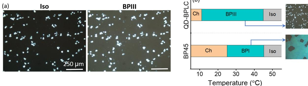
Fig. 2 (a) The POM images of QD-BPLC (kept between crossed polarizers,  $\times 10$  POL quality objective) captured while cooling the sample from Iso show the foggy background in BPIII and the dark field of view in Iso against bright scattering QDs. (b) The phase sequence of the BP45 and QD-BPLC mixtures depicting the blue phase thermal range enhancement and transformation of BPI to BPIII in the presence of QDs.
