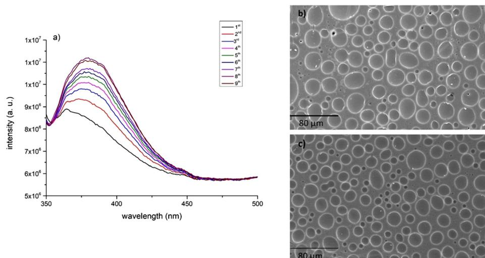
Fig. 16 (a) Emission spectra of  $C_2mimCl@PSU$  upon successive irradiations (1st–9th) at 314 nm (b) SEM images of  $C_2mimCl@PSU$  before irradiation (c) SEM images of  $C_2mimCl@PSU$  after irradiation at 314 nm.
