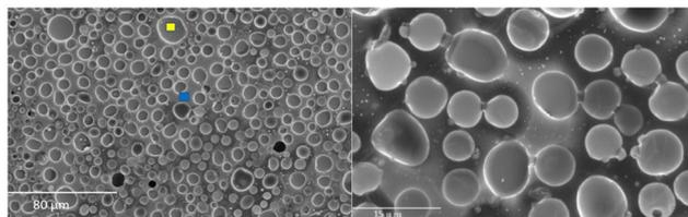
Fig. 12 Morphology of  $[C_2mim][fod]@PSU$  with 7% loading with agglomerates (yellow square) with spherical shape and film background in the blue square (left image). Magnification showing neck-shaped bonds between the drops (right image).
