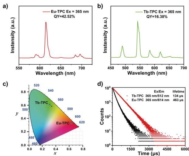
Fig. 2 Normalized luminescence spectra of (a) Eu-TPC and (b) Tb-TPC in the crystal state at room temperature.  $\lambda_{\text{ex}} = 365$  nm. (c) CIE 1931 chromaticity coordinates of Eu-TPC and Tb-TPC. (d) Time-resolved luminescent spectra of Eu-TPC and Tb-TPC at room temperature.  $\lambda_{\text{ex}} = 365$  nm.
