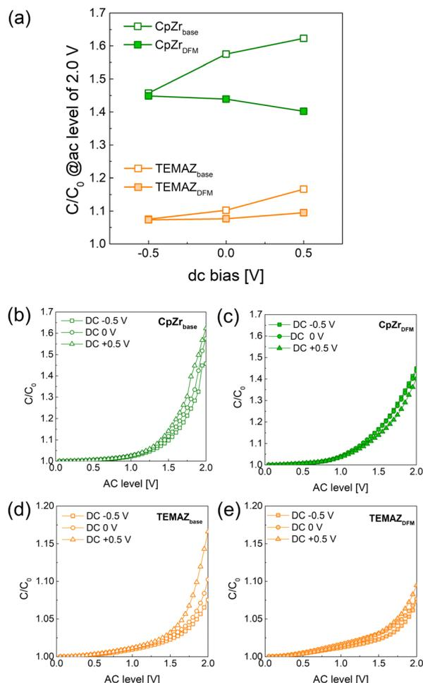
Fig. 5 (a) Relative capacitance density ( $C/C_0$ , where  $C_0$  denotes the capacitance at the AC level of 0 V) at the AC level of 2.0 V with respect to the DC bias varied by employing precursors and sequences;  $C/C_0$  vs. AC level plot with DC bias of  $-0.5$ ,  $0$ , and  $0.5$  V for (b)  $\text{CpZr}_{\text{base}}$ , (c)  $\text{CpZr}_{\text{DFM}}$ , (d)  $\text{TEMAZ}_{\text{base}}$ , and (e)  $\text{TEMAZ}_{\text{DFM}}$ . The thickness of  $\text{ZrO}_2$  was 10 nm for all samples.
