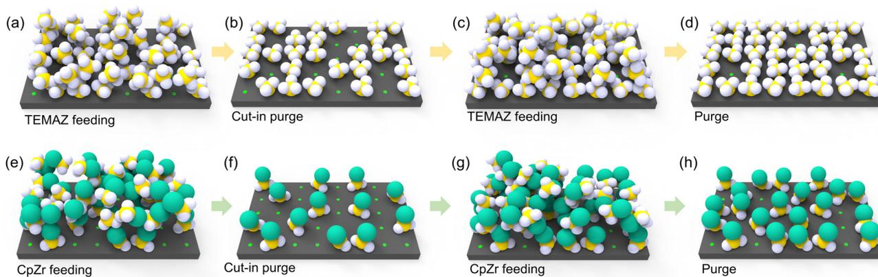
Fig. 4 Schematic diagram for depicting the precursor feeding procedure of TEMAZ<sub>base</sub> (a and b), TEMAZ<sub>DFM</sub> (a–d), CpZr<sub>base</sub> (e–f) and CpZr<sub>DFM</sub> (e–h) in the ZrO<sub>2</sub> ALD process.
