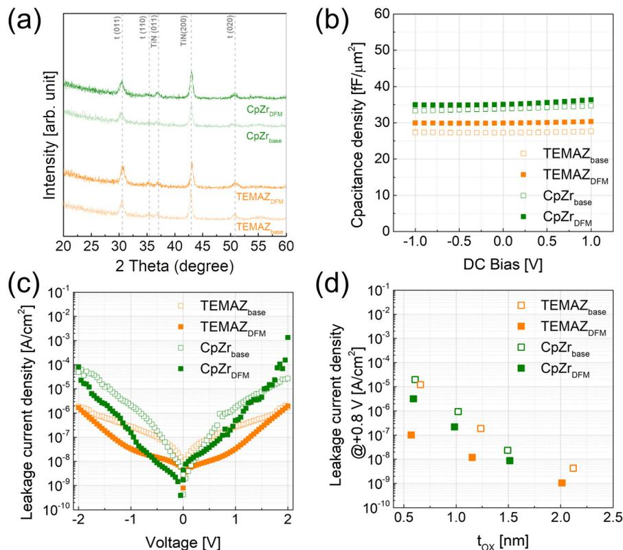
Fig. 7 (a) XRD patterns, (b) capacitance density vs. DC bias curves, and (c) leakage current density vs. applied bias curves for the 10 nm-thick-ZrO<sub>2</sub> thin films; and (d)  $J$ - $t_{\text{ox}}$  plot for the ZrO<sub>2</sub> thin films for varied physical thickness.
