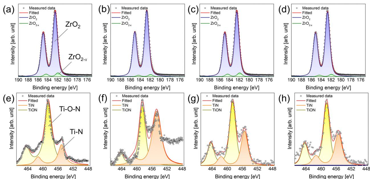
**Fig. 3** XPS spectra of (a)–(d) Zr 3d and (e)–(h) Ti 2p of  $\text{ZrO}_2$  thin film deposited on TiN substrate using (a), (e)  $\text{TEMAZ}_{\text{base}}$ , (b) and (f)  $\text{TEMAZ}_{\text{DFM}}$ , (c) and (g)  $\text{CpZr}_{\text{base}}$ , and (d) and (h)  $\text{CpZr}_{\text{DFM}}$ .
