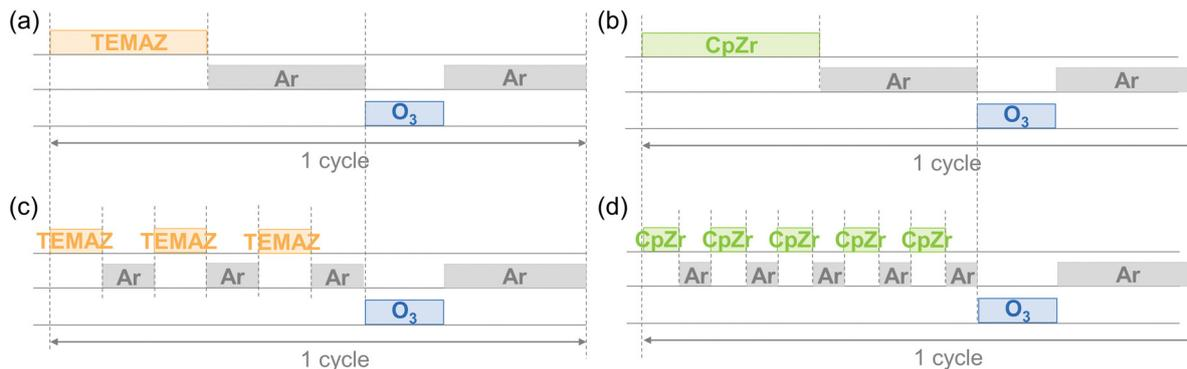
Fig. 1 Schematic of the ALD process sequences of base sequence with (a) TEMAZ (TEMAZ<sub>base</sub>), (b) CpZr (CpZr<sub>base</sub>), and DFM sequence with (c) TEMAZ (TEMAZ<sub>DFM</sub>), (d) CpZr (CpZr<sub>DFM</sub>).
