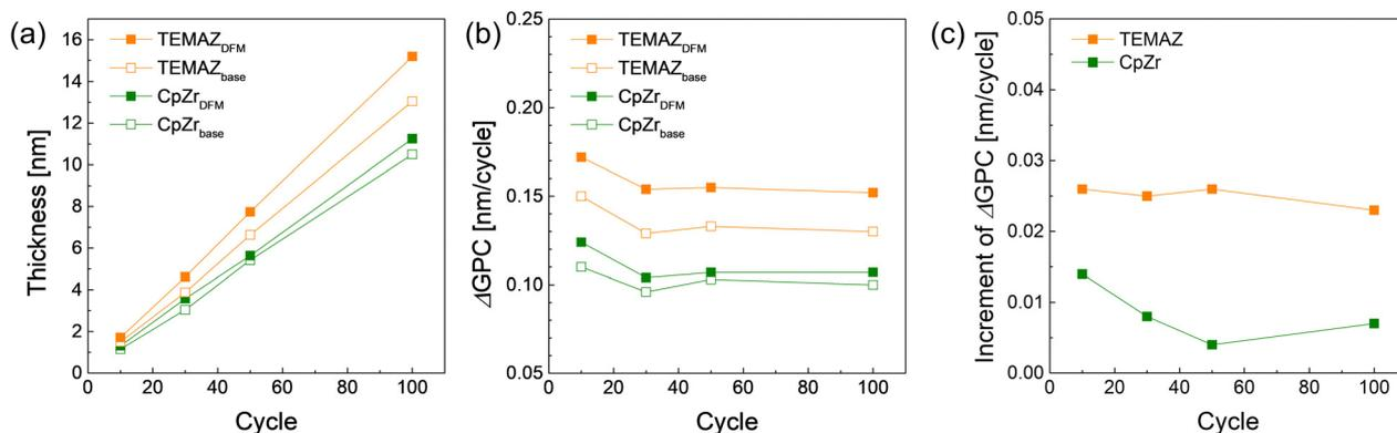
Fig. 2 (a) ZrO<sub>2</sub> thin film thickness, (b) differential growth rate ( $\Delta$ GPC), and (c) increment of growth rate with respect to the cycle number varied by employing precursors and sequence.
