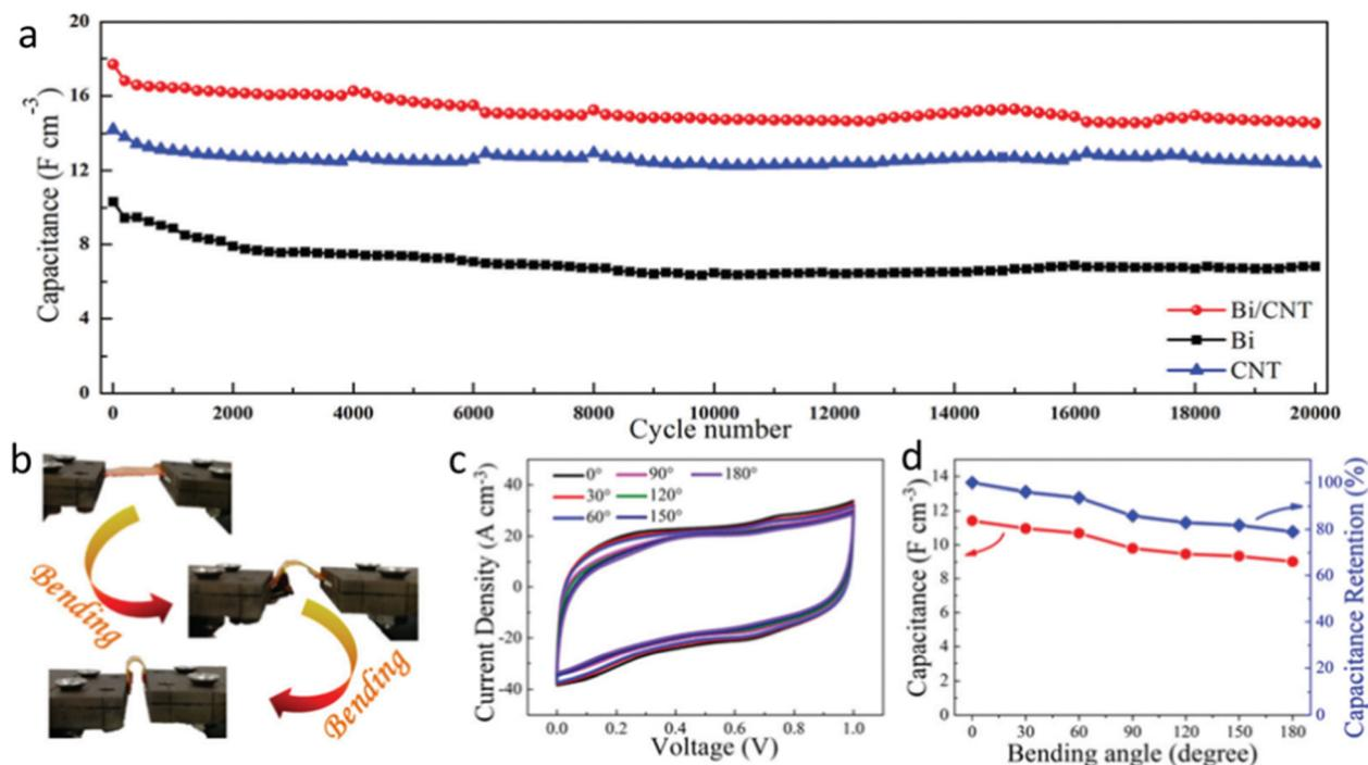
Fig. 10 (a) Cycling performance of capacitance for Bi/CNTs, Bi and CNTs at a scan rate of  $0.5 \text{ V s}^{-1}$ . (b) Photographs of Bi/CNTs tested under different bending angles. (c) CV curves obtained at different bending angles, at  $0.5 \text{ V s}^{-1}$ . (d) Volumetric capacitance and capacitance retention as a function of bending angle. Reprinted with permission from RSC.<sup>106</sup>
