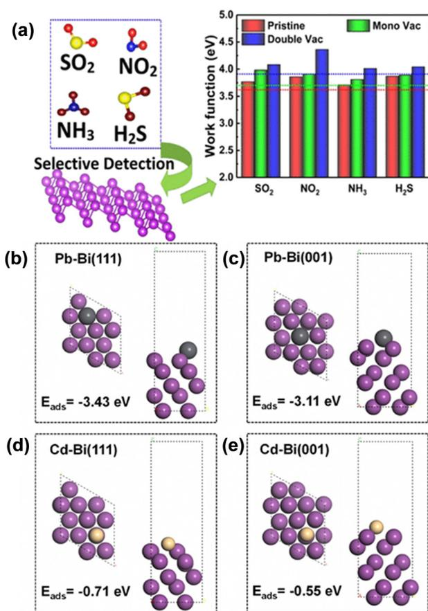
Fig. 7 (a) Sensing of  $\text{SO}_2$ ,  $\text{NO}_2$ ,  $\text{NH}_3$ , and  $\text{H}_2\text{S}$  gas using bismuthene. Reprinted with permission from ACS.<sup>85</sup> Adsorption energies and adsorption configurations of lead on (b) Bi-ene and bismuth nanosheets (c) and cadmium on Bi-ene (d) and (e) bismuth nanosheets, respectively (black, yellow and violet balls represent Pb, Cd and Bi atoms, respectively). Reprinted with permission from Elsevier.<sup>86</sup>
