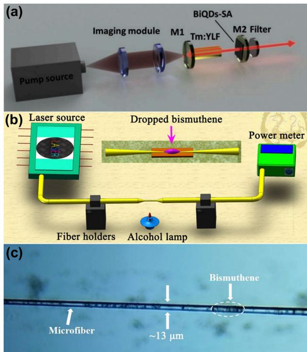
Fig. 9 (a) Schematic of Q-switched laser cavity based on bismuthene quantum dots. Reprinted with permission from Elsevier.<sup>78</sup> (b) Schematic diagram of the experimental setup for the fabrication of a microfiber. Reprinted with permission from ACS Publications.<sup>96</sup> (c) Microscopy image of the prepared microfiber saturable absorber based on bismuthene. Reprinted with permission from ACS Publications.<sup>96</sup>
