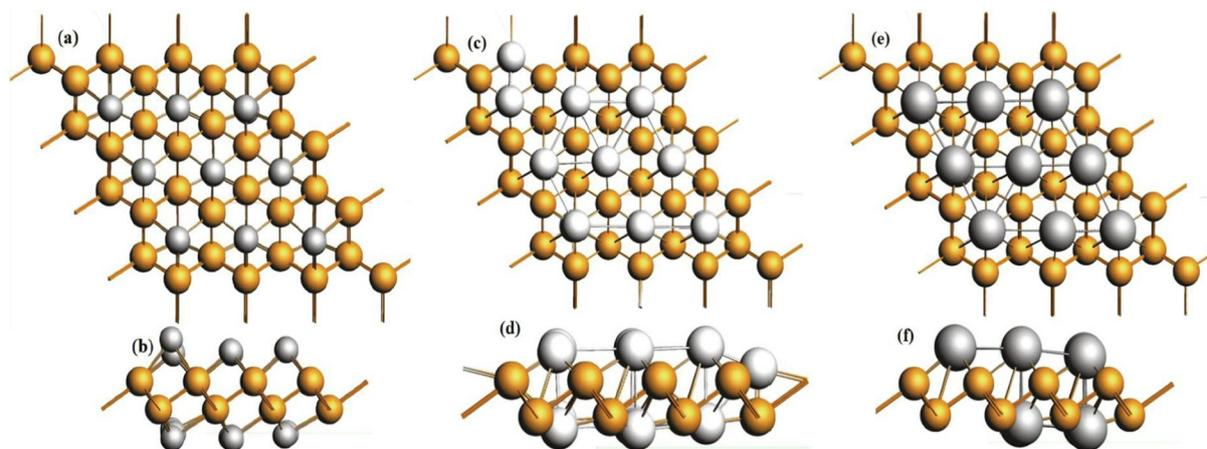
Fig. 11 Fully lithiated, sodiated and potassiated b-Bi structures from z-axis (a, c and e) and x-axis (b, d and f) views, respectively. Reprinted with permission from Elsevier.<sup>108</sup>
