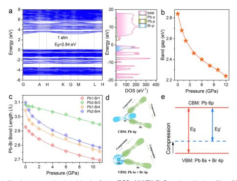
Fig. 4 (a) DFT calculated band structures and projected density of states (DOS) of (HMTA)<sub>3</sub>Pb<sub>2</sub>Br<sub>7</sub> under ambient conditions. (b) Calculated band gap evolution of (HMTA)<sub>3</sub>Pb<sub>2</sub>Br<sub>7</sub> under high pressure. (c) Calculated Pb-Br bond length evolution as a function of pressure. (d) Models of band gap narrowing upon compression. (e) Diagram of the VBM and CBM evolution upon compression.
