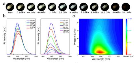
Fig. 1 (a) High-pressure optical PL micrographs of the (HMTA)<sub>3</sub>Pb<sub>2</sub>Br<sub>7</sub> crystal. (b) PL spectra of the (HMTA)<sub>3</sub>Pb<sub>2</sub>Br<sub>7</sub> crystal measured under different pressures. (c) Two-dimensional projection of the PL spectra under high pressure.
