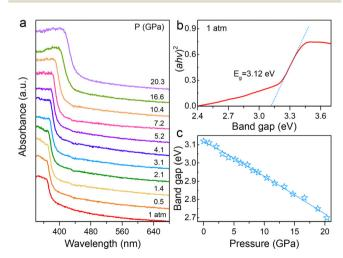
Fig. 2 (a) Evolution of the UV-Vis absorption spectra of the (HMTA)<sub>3</sub>Pb<sub>2</sub>Br<sub>7</sub> crystal at selected pressures. (b) The Tauc plot of (HMTA)<sub>3</sub>Pb<sub>2</sub>Br<sub>7</sub> under ambient conditions. (c) Demonstration of the band-gap narrowing in (HMTA)<sub>3</sub>Pb<sub>2</sub>Br<sub>7</sub> at high pressures.
