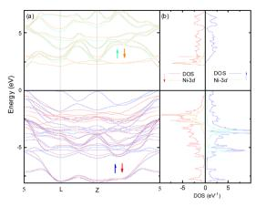
Fig. 2 Calculated electronic structure of NiGa<sub>2</sub>S<sub>4</sub>. (a) Band structure along principal directions of the first Brillouin zone. (b) Density of states (DOS) for the spin-up ( $\uparrow$ ) and spin-down ( $\downarrow$ ) channels including PDOS for Ni-3d states.
