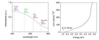
Fig. 5 (a) UV-Vis absorbance spectrum of an exfoliated NiGa<sub>2</sub>S<sub>4</sub> DMF suspension. The wavelength of the LED light source employed for the PEC study is marked by dashed lines. (b) Tauc plot used to extract the optical band gap of NiGa<sub>2</sub>S<sub>4</sub> nanosheets.
