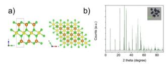
Fig. 1 Crystalline structure of hexagonal NiGa<sub>2</sub>S<sub>4</sub> along the c-axis and the ab plane. (b) XRD pattern of NiGa<sub>2</sub>S<sub>4</sub> crystalline powder. In the inset a sample of the crystals obtained via CVT synthesis is shown. The indexed XRD pattern of the NiGa<sub>2</sub>S<sub>4</sub> crystals and powders are shown in Fig. S1 and
