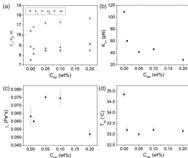
Fig. 7 Dependence of the physical properties on the particle concentration  $C_{NP}$  for the PLPSLC composites: (a) the dielectric constants  $\epsilon_{\parallel}$  and  $\epsilon_{\perp}$  and dielectric anisotropy  $\Delta\epsilon$ , (b) the splay elastic constant  $K_{11}$ , (c) the viscosity  $\gamma_1$ , (d) the nematic-isotropic transition temperature  $T_{NI}$ . All measurements, except those of  $T_{NI}$ , were taken at  $T = 29^{\circ}\text{C}$ ,  $f = 1$  kHz.
