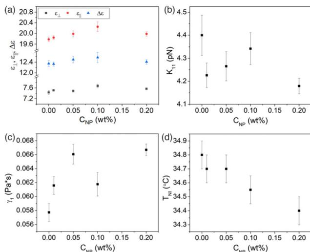
**Fig. 3** Dependence of the physical properties on the particle concentration  $C_{NP}$  for the PLLC composites: (a) the dielectric constants  $\varepsilon_{\parallel}$  and  $\varepsilon_{\perp}$  and dielectric anisotropy  $\Delta\varepsilon$ , (b) the splay elastic constant  $K_{11}$ , (c) the viscosity  $\gamma_1$ , (d) the nematic–isotropic transition temperature  $T_{NI}$ . All measurements, except those of  $T_{NI}$ , were taken at  $T = 29$  °C,  $f = 1$  kHz.
