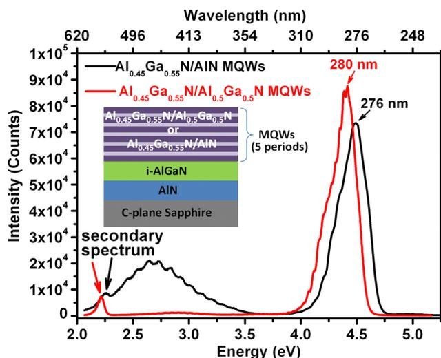
Fig. 2 PL spectra of both Al<sub>0.45</sub>Ga<sub>0.55</sub>N/AlN MQWs and Al<sub>0.45</sub>Ga<sub>0.55</sub>N/Al<sub>0.5</sub>Ga<sub>0.5</sub>N MQWs. The inset shows their epitaxial structures.
