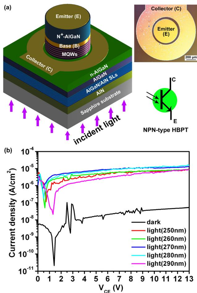
Fig. 4 (a) Schematic configuration, physical image and symbol of the NPN-type AlGaN-based HBPT. (b) The  $I$ – $V$  characteristic curves of the device measured in the dark and under different illumination wavelengths using a semi-log scale.
