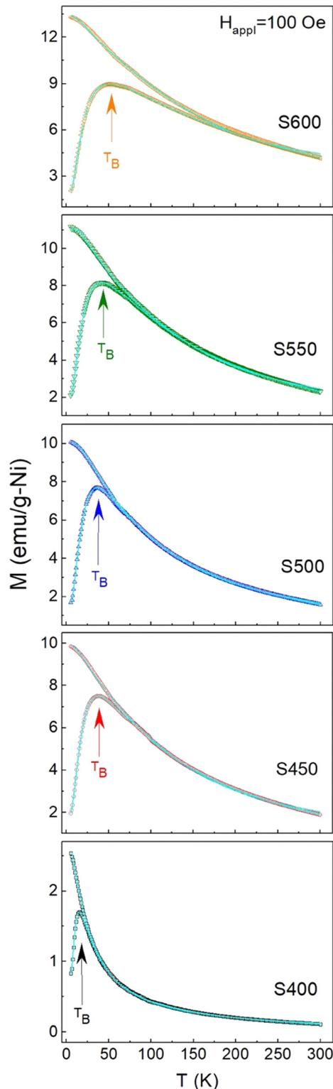
**Fig. 11**  $M(T)$  curves measured in the ZFC and FC regime under an applied magnetic field,  $H_{\text{appl}} = 100$  Oe. The dots correspond to the experimental data, while the solid line is associated with the Stoner–Wohlfarth-based fit. Arrows point out the average blocking temperatures ( $T_B$ ). (see text for details).
