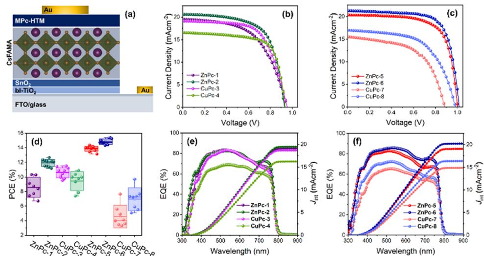
Fig. 6 Proposed device architecture: fluorine-doped tin oxide (FTO)/bi-TiO<sub>2</sub>/SnO<sub>2</sub>/perovskite/MPc/Au (a),  $J$ - $V$  curves of the device using (b) symmetric MPcs and (c) asymmetric MPcs, (d) statistical PCE of PSCs with different MPc-HTMs, corresponding IPCE and integrated current density ( $J_{\text{int}}$ ) of the device with (e) symmetric MPcs and, (f) asymmetric MPcs.
