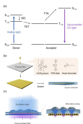
Fig. 1 (a) Typical mechanism of TTA-UC. (b) Schematic illustration of porous film impregnation method using Ir(C6)<sub>2</sub>(acac), TIPS-Nph, and hexyl benzoate as a donor, acceptor and solvent, respectively. (c) Schematic illustration of integrating a porous film with a microlens array.
