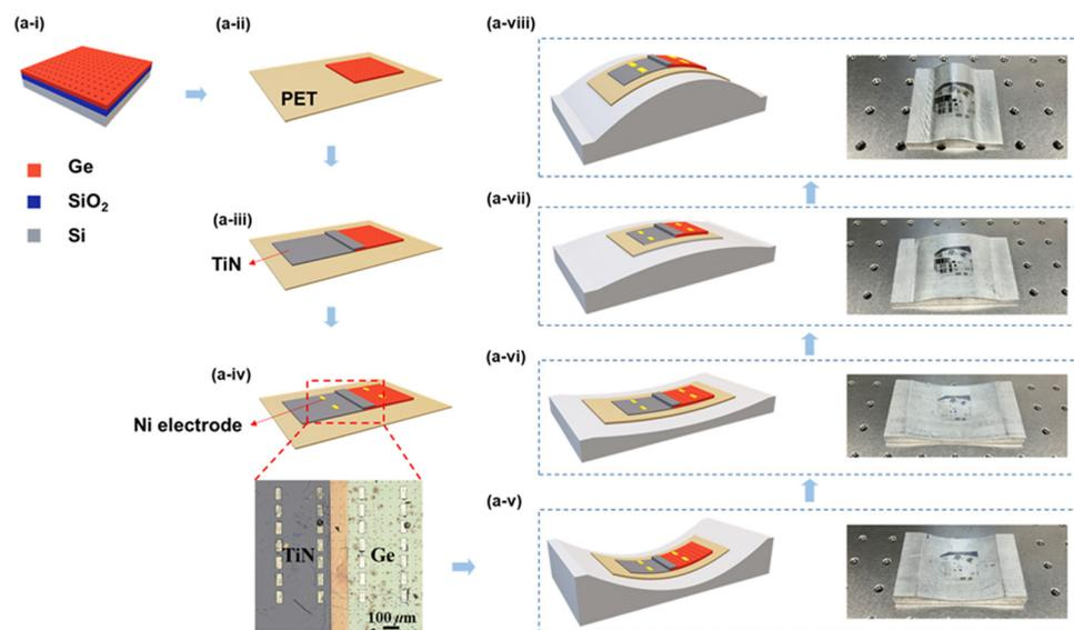
**Fig. 1** Fabrication process of flexible TiN/Ge PDs and strain modulation by applying external strain. Schematic illustration of (a-i) patterned GeOI by dry etching, (a-ii) Ge NM transferred on PET substrates, followed by (a-iii) TiN deposition, and (a-iv) Ni electrode deposition and the microscopic image of the fabricated TiN/Ge PDs. (a-v–viii) Application of compressive and tensile strain to the devices.
