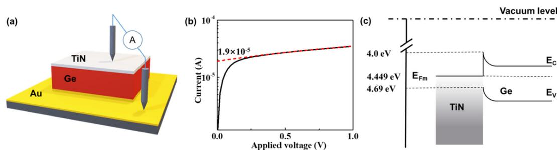
Fig. 2 (a) Schematic of the TiN/Ge Schottky diode and  $I$ – $V$  measurement to extract the SBH between Ge and TiN. (b)  $I$ – $V$  curve of the TiN/Ge Schottky diode. The red dashed line shows the saturation current. (c) Band diagram of the TiN/Ge heterojunction.
