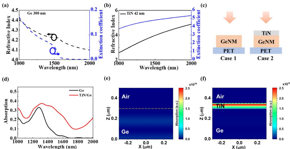
Fig. 3 Refractive index and extinction coefficient of (a) Ge and (b) TiN in the wavelength range of 1 to 2  $\mu\text{m}$ . (c) Schematic cross-sectional structure of the Ge PD (case 1) and TiN/Ge PD (case 2). (d) Simulated light absorption plots of the TiN/Ge junction and Ge from 1 to 2  $\mu\text{m}$ . Simulated light absorption of cross-sectional maps of (e) Ge and (f) interfaces at TiN/Ge. The wavelength of incident light in the simulation is 1.5  $\mu\text{m}$ .
