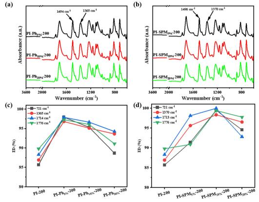
Fig. 2 FTIR spectra of (a) (PhNH<sub>2</sub>/ODA)/PMDA co-PI films cured at 200 °C and (b) (SPMNH<sub>2</sub>/ODA)/PMDA co-PI films cured at 200 °C and trend of different IDs of (c) (PhNH2/ODA)/PMDA co-PI films cured at 200 °C and (d) (SPMNH2/ODA)/PMDA co-PI films cured at 200 °C.
