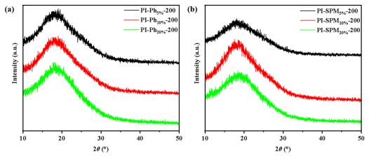
Fig. 3 XRD patterns of (a) (PhNH<sub>2</sub>/ODA)/PMDA co-PI films cured at 200 °C and (b) (SPMNH<sub>2</sub>/ODA)/PMDA co-PI films cured at 200 °C
