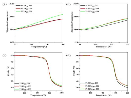
Fig. 4 TMA curves of (a) (PhNH<sub>2</sub>/ODA)/PMDA co-Pl films and (b) (SPMNH<sub>2</sub>/ODA)/PMDA co-Pl films; TGA curves of (c) (PhNH<sub>2</sub>/ODA)/PMDA co-Pl films and (d) (SPMNH2/ODA)/PMDA co-PI films
