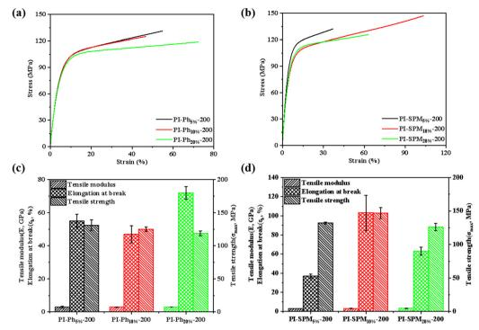
Fig. 5 Typical stress-strain curves of (a) (PhNH<sub>2</sub>/ODA)/PMDA co-PI films and (b) (SPMNH<sub>2</sub>/ODA)/PMDA co-PI films and detailed data of mechanical properties of (c) (PhNH<sub>2</sub>/ODA)/PMDA co-PI films and (d) (SPMNH<sub>2</sub>/ODA)/PMDA co-PI films.
