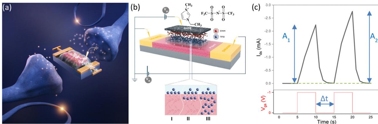
**Fig. 1** (a) Bio-inspired synaptic IGT transistor. (b) Device scheme and possible doping regimes (I to III) upon application of a negative  $V_{gs}$  to a P3HT-based IGT; molecular structures of the ions constituting the ionic liquid employed as gating medium in this study. (c) A pair of successive  $V_{gs}$  inputs ( $-1$  V) for 5 s with a pulse interval  $\Delta t = 5$  s applied to an IGT.  $A_1$  and  $A_2$  are the amplitudes of the drain-source current ( $I_{ds}$ ).
