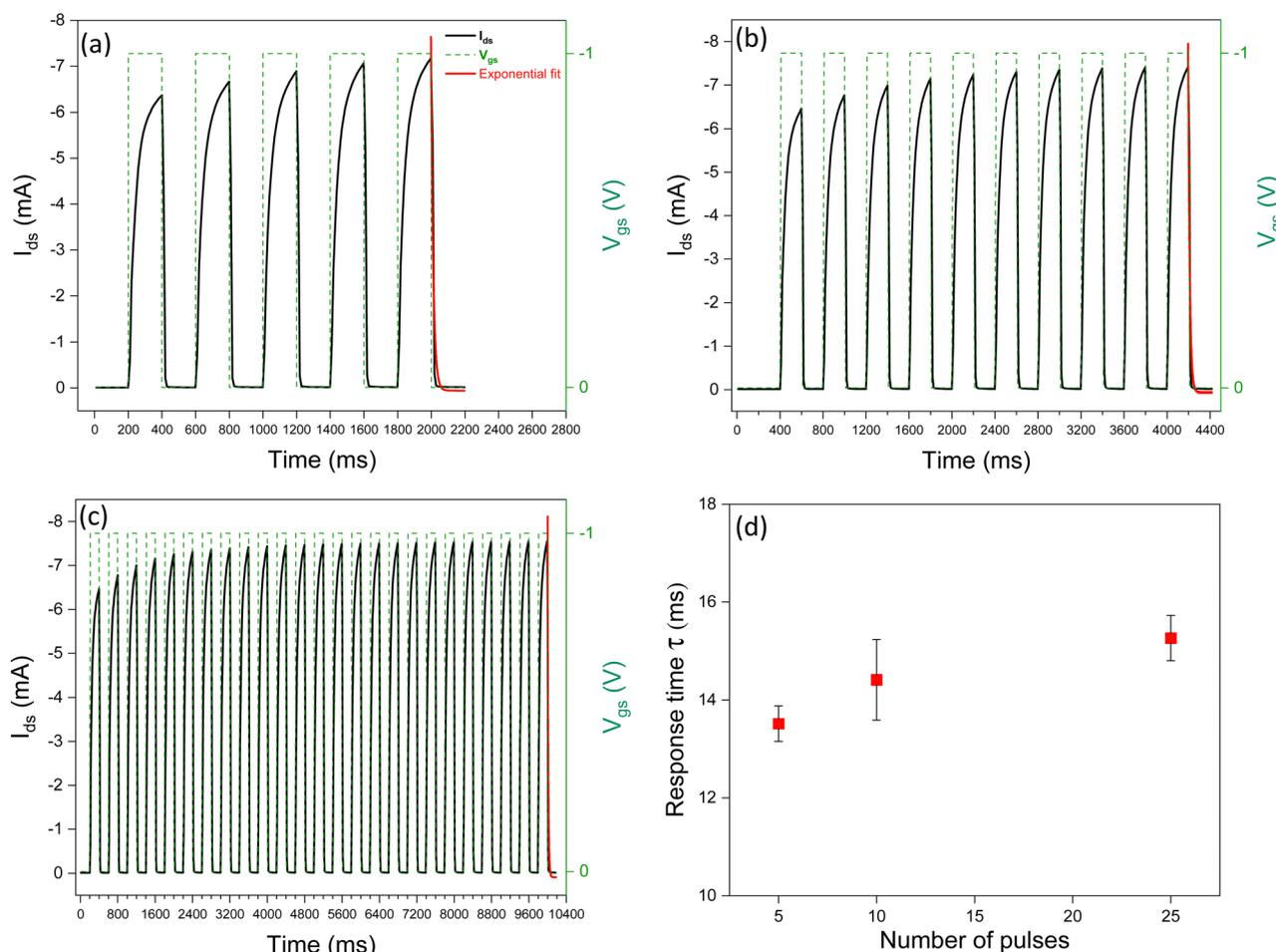
Fig. 3 Transient  $I_{ds}$  response of [EMIM][TFSI]-gated P3HT transistors in response to different numbers of  $V_{gs}$  square step train pulses.  $V_{gs} = -1$  V at  $V_{ds} = -0.6$  V (a) 5 pulses, (b) 10 pulses, (c) 25 pulses. (d) Response time versus number of  $V_{gs}$  pulses. The duration and interval of each  $V_{gs}$  pulse is 200 ms; exponential fits used to estimate the response time are in red.
