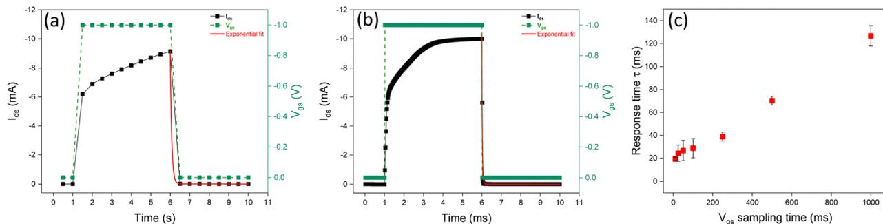
Fig. 5 Transient response of an [EMIM][TFSI]-gated P3HT transistor at different  $V_{gs}$  pulse sampling times: (a) 500 ms, (b) 25 ms; the duration of  $V_{gs}$  pulse is 5 s. (c) Response time versus different  $V_{gs}$  sampling times (10, 25, 50, 100, 200, 500, and 1000 ms) at  $V_{ds} = -0.8$  V.
