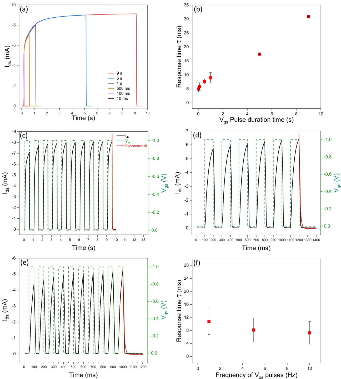
Fig. 4 (a) and (b) Transient  $I_{ds}$  characteristic response of an [EMIM][TFSI]-gated P3HT transistor versus different duration times. Transient response of transistors in response to  $V_{gs}$  pulses with different frequencies (c) 1 Hz, (d) 5 Hz, and (e) 10 Hz. (f) Response time versus frequency of  $V_{gs}$  pulses ( $V_{gs} = -1$  V, at  $V_{ds} = -0.6$  V).
