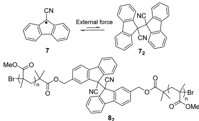
Fig. 5 The equilibrium between cyanofluorene radical (**7**) and its dimer difluorenylsuccinonitrile (**7<sub>2</sub>**) and the example of a polymer bearing cyanofluorene radical (**8<sub>2</sub>**).
