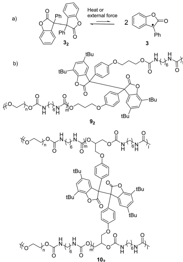
Fig. 6 (a) The equilibrium between benzofuranone radical (3) and its dimer (3<sub>2</sub>); (b) examples of polymers bearing the benzofuranone radical (9<sub>2</sub> and 10<sub>2</sub>).
