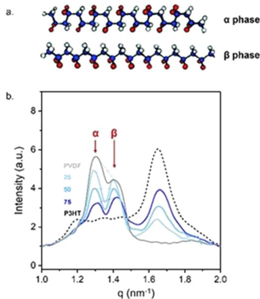
Fig. 3 Relating intermixing with macroscopic film properties. (a) Schematic illustrations of the non-polar  $\alpha$  and polar  $\beta$  polymorphs of PVDF.<sup>39</sup> (b) Grazing-angle wide-angle X-ray scattering in-plane intensity line-cuts of solution-processed P3HT:PVDF thin films ( $\approx 60 \text{ kg mol}^{-1} : 350 \text{ kg mol}^{-1}$ ), showing signatures characteristic of the polar  $\beta$  phase of PVDF becoming most intense for the most vitrified 75 : 25 P3HT:PVDF blend.
