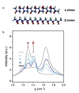
Fig. 3 Relating intermixing with macroscopic film properties. (a) Schematic illustrations of the non-polar  $\alpha$  and polar  $\beta$  polymorphs of PVDF. <sup>39</sup> (b) Grazing-angle wide-angle X-ray scattering in-plane intensity line-cuts of solution-processed P3HT:PVDF thin films ( $\approx$ 60 kg mol<sup>-1</sup>), showing signatures characteristic of the polar  $\beta$  phase of PVDF becoming most intense for the most vitrified 75:25 P3HT:PVDF blend.
