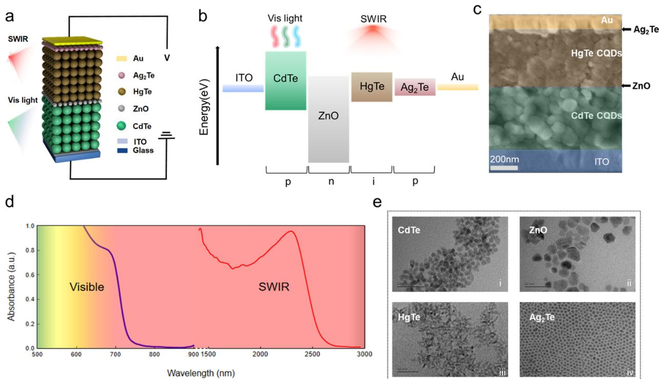
**Fig. 1** Architecture of the dual-band visible and SWIR photodetector. (a) Structure diagram of the dual-band device. (b) Energy band structure diagram of the dual-band device. (c) Cross-sectional SEM image of the dual-band device. (d) Absorption spectra of CdTe CQDs and HgTe CQDs. (e) TEM images of the CdTe, ZnO, HgTe, and Ag<sub>2</sub>Te materials.
