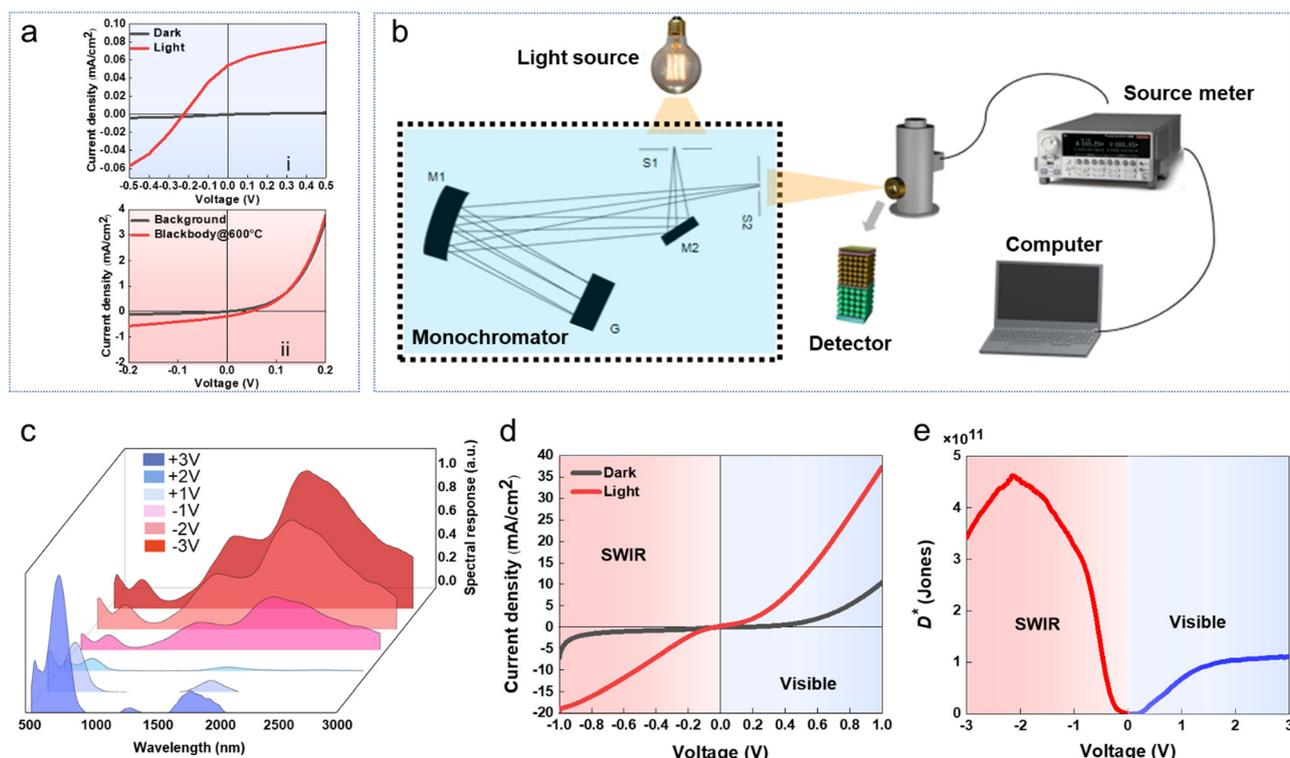
**Fig. 2** Performance of dual-band visible and SWIR photodetectors. (a) Current density–voltage curves of CdTe/ZnO single-band device and ZnO/HgTe/Ag<sub>2</sub>Te single-band device. (b) Illustration of the performance characterization system. (c) Response spectra of the dual-band device under positive and negative bias. (d) Current density–voltage curves of the dual-band device. (e) Specific detectivity of the dual-band device under positive and negative bias.
