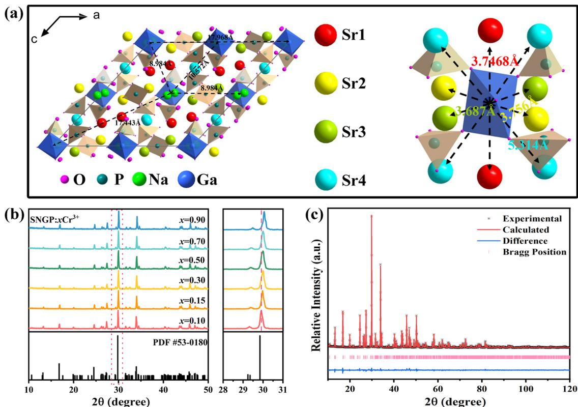
Fig. 1 (a) Crystal structure of the SNGP host; distances between adjacent  $\text{Ga}^{3+}$  ions, and distances between  $\text{Ga}^{3+}$  ions and  $\text{Sr}^{2+}$  ions. (b) XRD patterns of  $\text{SNGP}:x\text{Cr}^{3+}$  ( $x = 0.10, 0.15, 0.30, 0.50, 0.70,$  and  $0.90$ ) (c) Rietveld refinement of  $\text{SNGP}:0.15\text{Cr}^{3+}$  phosphors.
