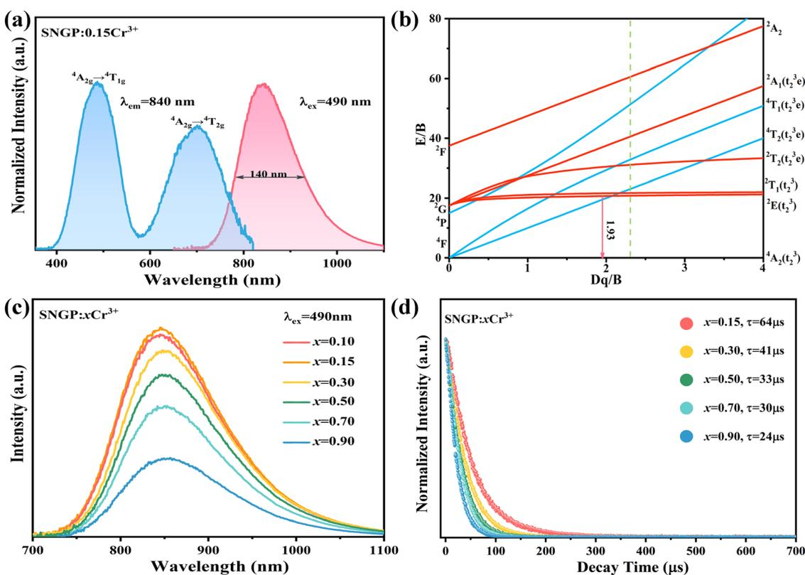
Fig. 3 (a) PLE and PL spectra of SNGP:0.15Cr<sup>3+</sup>. (b) Tanabe–Sugano diagram for Cr<sup>3+</sup> in an octahedral crystal field environment. (c) Relationship between concentration and emission intensity of the Cr<sup>3+</sup> ions in SNGP:*x*Cr<sup>3+</sup> (*x* = 0.10, 0.15, 0.30, 0.50, 0.70, and 0.90). (d) Decay curves of SNGP:*x*Cr<sup>3+</sup> (*x* = 0.15, 0.30, 0.50, 0.70, and 0.90).
