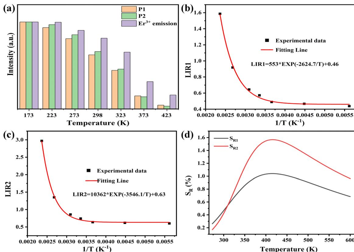
Fig. 11 (a) Histogram of the temperature-dependent emission intensity for P1, P2 and  $\text{Er}^{3+}$ -emission. (b) LIR 1 versus  $1/T$  (c) LIR 2 versus  $1/T$ . (d) Dependencies of  $S_{R1}$  and  $S_{R2}$  on temperature.
