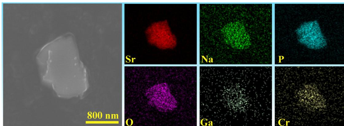
Fig. 2 SEM image and elemental maps of the SNGP:0.30Cr<sup>3+</sup> phosphor.
