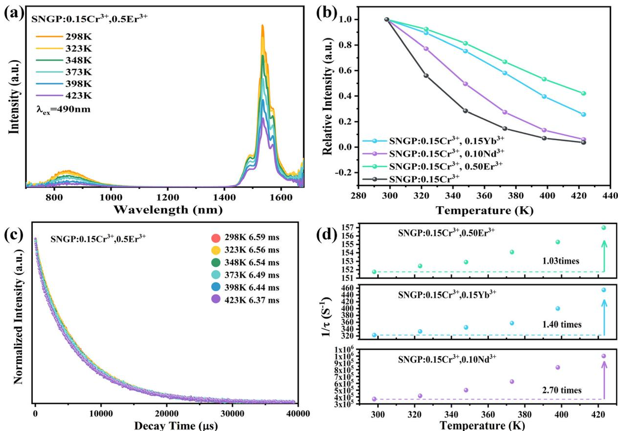
Fig. 7 (a) PL spectra of phosphor **4** at different temperatures. (b) Dependencies of PL intensities for phosphors **1–4** on temperature. (c) Decay curves of phosphor **4** at different temperatures. (d) Decay rates ( $1/\tau$ ) of the  $\text{Nd}^{3+}$ ,  $\text{Yb}^{3+}$  and  $\text{Er}^{3+}$  luminescence at different temperatures corresponding to phosphors **2–4**.
