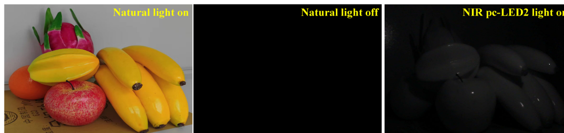
Fig. 9 Images of fruits illuminated with natural light and the NIR pc-LED 2 light.
