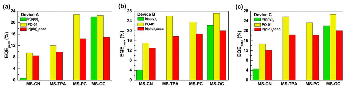
Fig. 7 Peak EQEs of the tested devices for different hosts and emitters: (a) A series; (b) B series; (c) C series.
