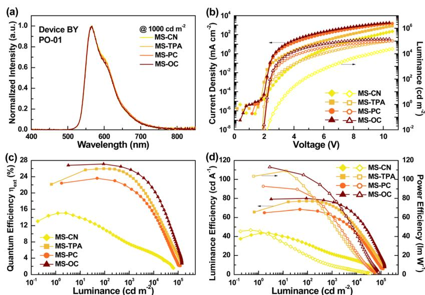
Fig. 8 (a) Normalized EL spectra at a luminance of 10<sup>3</sup> cd m<sup>-2</sup>; (b) current density–voltage–luminance (*J*–*V*–*L*) characteristics; (c) EQE vs. luminance; (d) luminance/power efficiency vs. luminance, for devices **BY1**, **BY2**, **BY3**, and **BY4**.
