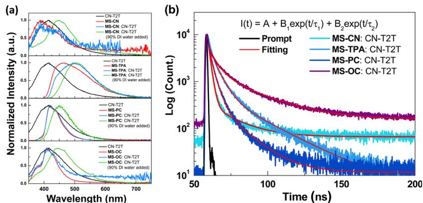
Fig. 4 (a) Normalized PL spectra of CN-T2T, the four synthesized materials and their mixtures in pure THF and with 90% water added. (b) Transient PL profiles of the mixture samples for THF with 90% water added.
