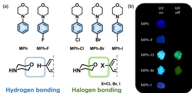
Fig. 1 (a) Chemical structures of MPh, MPh-F, MPh-Cl, MPh-Br and MPh-I. (b) Photographs taken before and after irradiation (365 nm) under ambient conditions.
