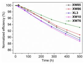
Fig. 7 Plots of the changes in the PCEs vs. the illumination time for the solar cells sensitized by XW85, XW86, XL3, XW10 and XW76, respectively.
