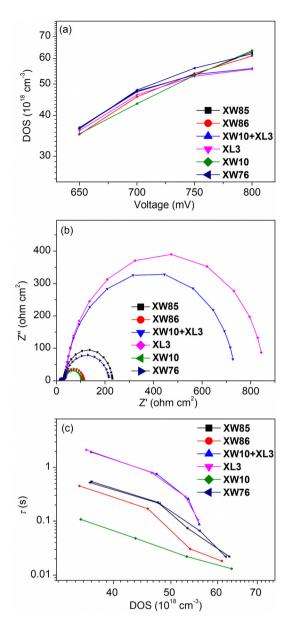
**Fig. 6** (a) Plots of DOS *versus* the bias voltages, (b) complex-plane plots at applied voltage of -0.75 V, and (c)  $\tau$  *versus* DOS of the DSSCs using  $\rm I_3^-/\rm I^-$  electrolyte measured in the dark.
