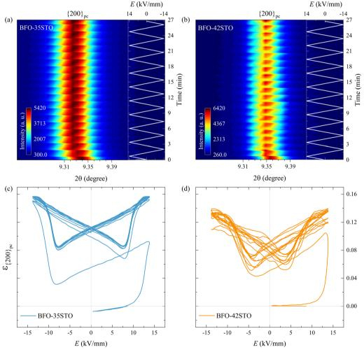
Fig. 7 Contour map of the  $\{200\}_{pc}$  reflections at  $\psi = 0^{\circ}$  under bipolar *E*-field cycling for (a) BFO-35STO, and (b) BFO-42STO. Lattice strain hysteresis loop for (c) BFO-35STO, and (d) BFO-42STO. In both compositions the  $\{200\}_{pc}$  peak remains unsplit during the entire field cycling.
