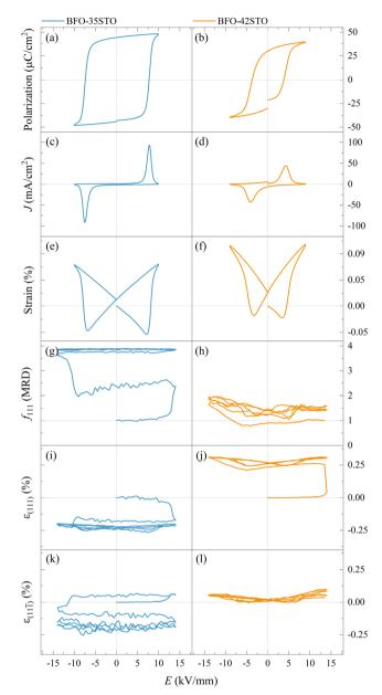
Fig. 6 Macroscopic P-E (a and b), J-E (c and d), and S-E (e and f) hysteresis loops,  $f_{111}$  texture indexes (g and h), and lattice strain for (111) (i and j), and (111) domains (k and l), for BFO-35STO and BFO-42STO, respectively. The cycles shown in (q-l) corresponds to the first two bipolar periods and is representative of the entire dataset.
