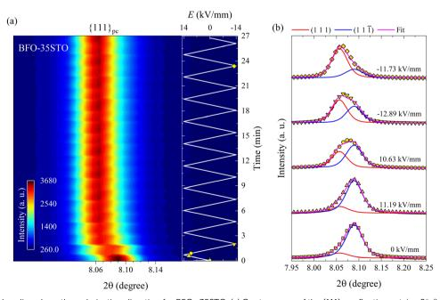
Fig. 2 Bipolar E-field cycling along the polarization direction for BFO-35STO. (a) Contour map of the  $\{111\}_{pc}$  reflections at  $\psi=0^{\circ}$ . (b) Deconvoluted peak fitting evolution for selected in situ diffracted intensity distributions. The insert in (a) represents the E(t) evolution, where the marked yellow symbols correspond to the fitted intensity distributions in (b).
