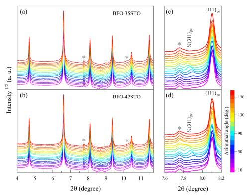
Fig. 1 Azimuthal angle-dependency of the XRD patterns for (a) BFO-35STO, and (b) BFO-42STO. The peaks marked with the star symbol (\*) belong to a minor secondary phase, most likely Sillenite ( $Bi_{25}FeO_{40}$ ). The panels (c and d) highlights the {111} $_{pc}$  and the 1/2{311} $_{pc}$  reflections for BFO-35STO and BFO-42STO, respectively.
