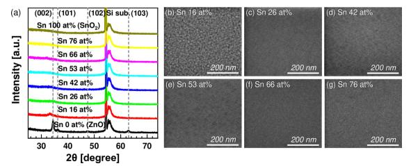
Fig. 1 (a) GIXRD patterns of ZnO, SnO<sub>2</sub>, and ZTO films with different Sn concentrations (as deposited). Planar SEM images of the ZTO films with (b) Sn 16 at%, (c) Sn 26 at%, (d) Sn 42 at%, (e) Sn 53 at%, (f) Sn 66 at%, (g) Sn 76 at%.
