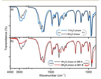
Fig. 3 ATR spectra recorded *in situ* following transformations: (a) from the initial  $1.11H_2O$  phase to the  $1.6H_2O$  phase and backward induced by a change in the humidity at room temperature; (b) from the  $1.6H_2O$  phase to the  $1.2H_2O$  phase and backward induced by a change in the temperature.
