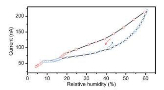
Fig. 4 Changes in the current response (conductivity) at 295 K and 1 V with an increase and a decrease in the relative humidity, induced by the reversible structural conversion of  $1.11H_2O$  to  $1.6H_2O$ .
