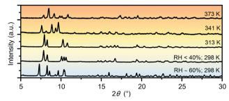
Fig. 2 PXRD patterns of the different hydrate phases and the dehydrated phase of the complex salt (TEA)<sub>4</sub>[V<sub>4</sub>O<sub>8</sub>(L-tart)<sub>2</sub>] (1) measured during heating and exposure to different relative humidities
