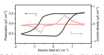
Fig. 5 Ferroelectric polarization at 295 K and RH < 5% for 1.6H<sub>2</sub>O showing P-E hysteresis loops and the corresponding current response at a 0.1 Hz switching frequency.
