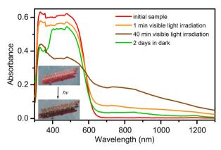
Fig. 7 Irradiation-time dependence of the UV-vis diffuse reflectance spectra of  $1.6H_2O$ . Spectra were recorded at 295 K ex situ at 0, 1 and 40 minutes of irradiation with a Xenon lamp (300 W, UV filter) and after a recovery period of 2 days in the dark.
