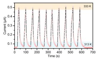
Fig. 6 Current response of the 1.5H2O phase at 10 V while switching between two heating stages at 313 K and at 333 K.
